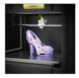
**Figure 1.30** Prototype model made with 3-D printing Real model of a shoe created with a rapid prototyping system.
