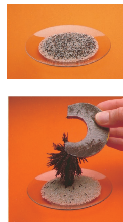
Figure 1.6 An example of separation based on differences in physical properties. Magnetic iron is separated from nonmagnetic substances. A large-scale version of this process is important in the recycling industry.
