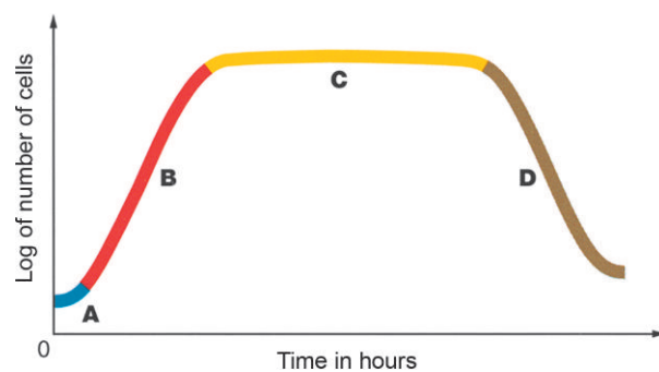
FIG. 1.3 Typical growth curve for a pure culture of bacteria. A=lag period, B=exponential phase, C=stationary phase, D=death phase. (From Pollution Science © 1996, Academic Press, San Diego, CA.)
