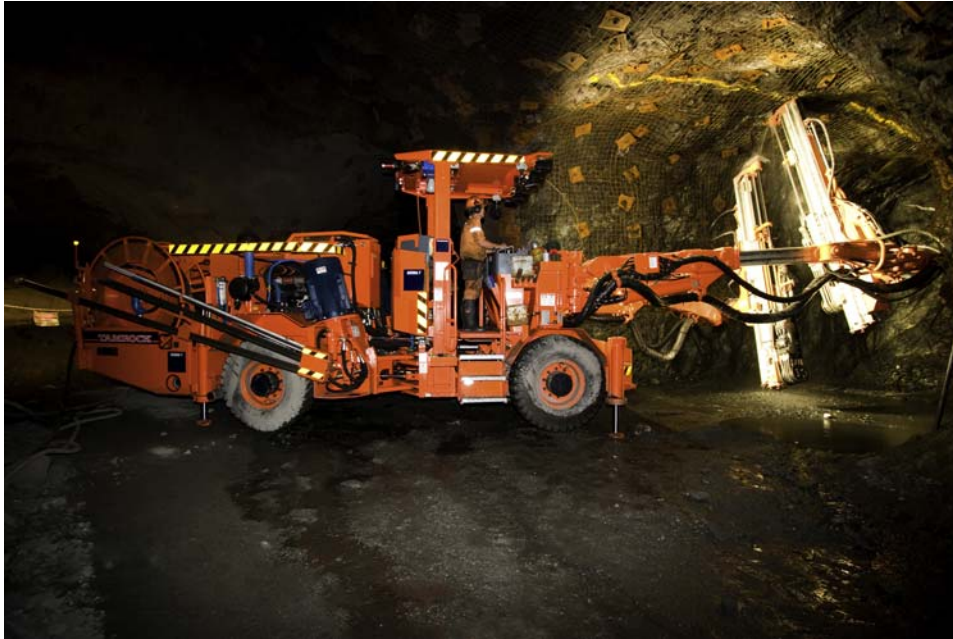
Figure 1.2 Underground mining operation. Underground mine showing wheeled mining machine. The drills on the right end of the vehicle are drilling up into the ore body. The drilled holes are subsequently filled with explosive which, when detonated, break the ore and drop the ore pieces onto the mine floor. The ore pieces are then elevated to the mine surface where they are crushed and sent to processing. A new mine in Arizona contains \sim 1.5\% Cu, 0.04\% Mo in chalcopyrite and molybdenite minerals. \sim 120 kilotonnes per day of this ore will be mined \sim 2300 m below ground level. About one-fourth of the world's mined copper is obtained by underground mining; the remainder is by surface mining. (Purchased from Roslyn Budd: www.buddphotography.com.au ).
