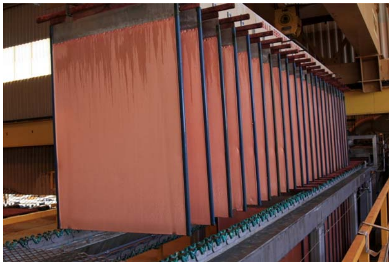
Figure 1.10 Plates of electrowon copper on stainless-steel cathodes after removal from an electrowinning cell. These cathodes are \sim 1 m wide and 1.3 m deep. They are carefully washed to remove electrolyte. The copper plates are then stripped off in automatic machines and sent to market. They typically contain <20 parts per million impurities. Note the polymer side strips—they prevent copper from plating around the edges. (Photograph courtesy of Freeport-McMoRan Copper & Gold Inc.)
