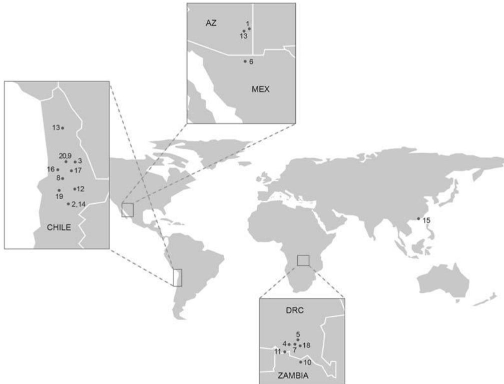
Figure 2.8 Map showing the locations of the world's 20 largest copper solvent extraction—electrowinning plants. Most of these are in Chile and the African Copper Belt. The numbers refer to the data in Table 2.6.
