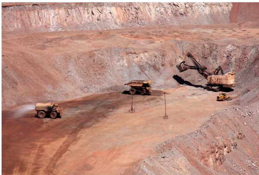
Figure 1.1 Open pit Cu mine. Note the new blast holes, top right, and blasted ore to the left of them. The shovel is placing blasted ore in the truck from where it will go to processing. The water truck is suppressing dust. The front-end loader is cleaning up around the shovel. The shovel is electric. Its insulated power wire mostly lies on the surface except over the wire bridge under which all vehicles travel to and from the shovel. (Photograph courtesy of Freeport—McMoRan Copper & Gold Inc.).
