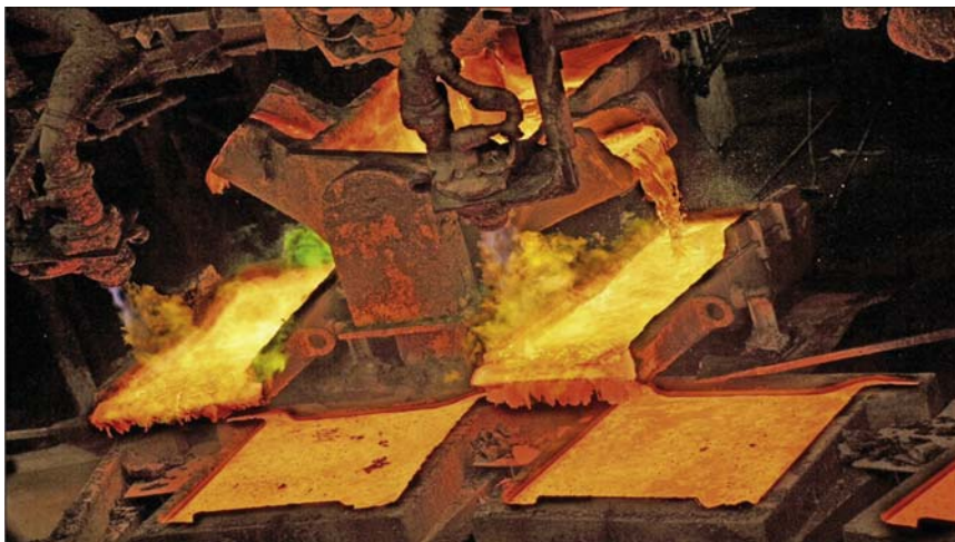
Figure 1.8 Casting of anodes for electrorefining. (Photo courtesy of Miguel Palacios.).
