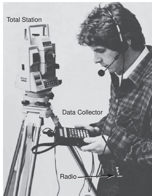
FIGURE 1.6 Sokkia total station.
