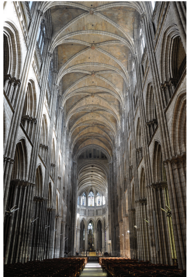
FIGURE 1.4 The groin vaults of the magnificent Rouen cathedral in northern France are an expression of a “correct” structure. Here, stone is used to its best ability in compression, with little or no tensile stresses being developed. The stone arches of the groin vault roof effectively channel the heavy load of the stone roof out and down to the exterior walls, where further structures on the exterior known as flying buttresses counteract the outward push.
