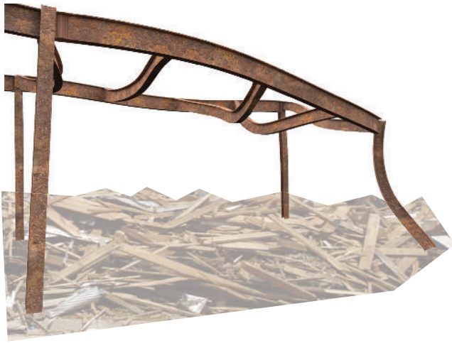
Figure 3.12 Warping of steel due to fire
