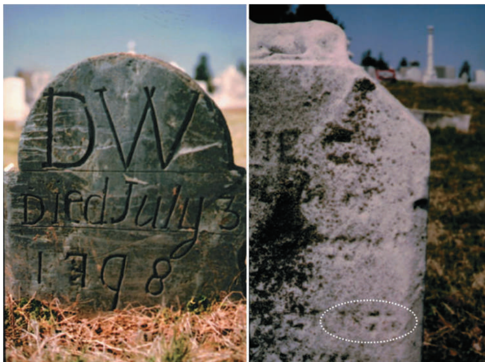
Figure 2.1 Two stone markers, photographed on the same day in the same cemetery, illustrate the effect of rock type on weathering rates. The date and initials carved in the slate marker in 1798 are still sharp and clear, while the date and figure of a lamb carved in the marble marker in 1875 have weathered almost beyond recognition. The slate rock consists largely of resistant silicate clay minerals, whereas the marble consists mainly of calcite, which is much more easily attacked by acids in rainwater. (Photos courtesy of Ray R. Weil)
