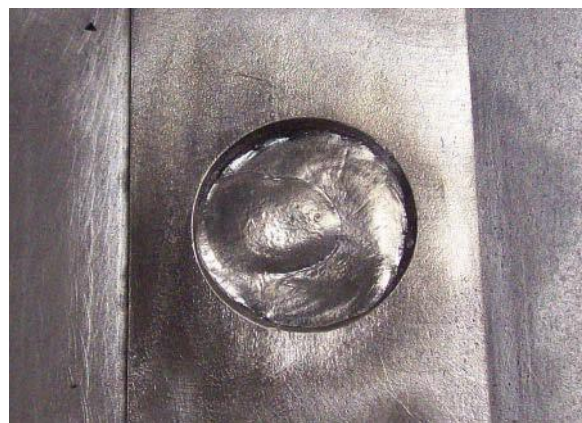
TYPICAL PLUG WELD
