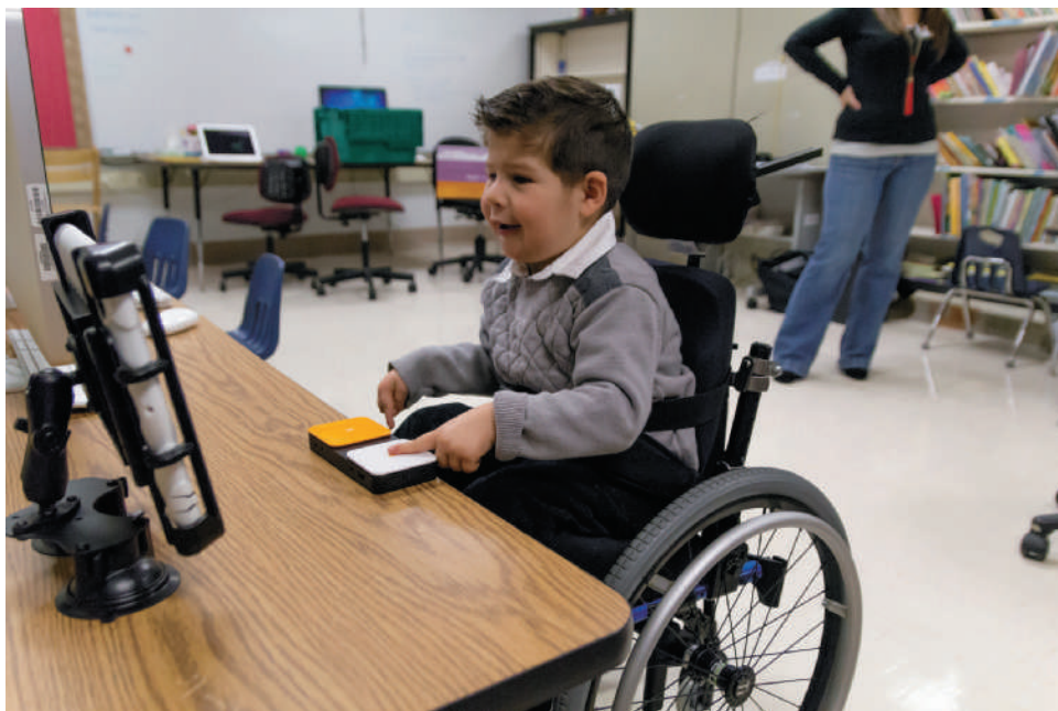
FIGURE 1.7 This child who has physical disabilities is accessing an iPad using a Bluetooth switch. The iPad is mounted securely on a stand because he is not able to hold it.
