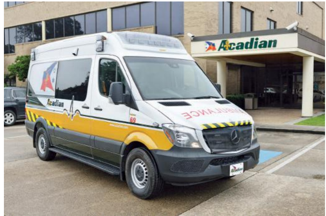
FIGURE 2-17 The diesel, unibody ambulance is becoming increasingly popular because of cost, fuel economy, and safety.
