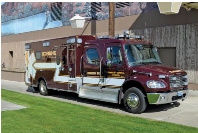
FIGURE 2-16 Some EMS systems have elected to use medium-duty ambulances that are built on a commercial truck chassis.
