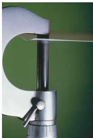
FIGURE 1–8 Example 1–6. Micrometer used for measuring small thicknesses.
