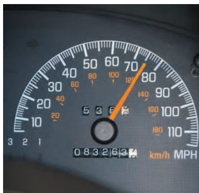
FIGURE 2-8 Car speedometer showing mi/h in white, and km/h in orange.
