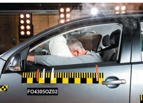
FIGURE 2–20 Example 2–11. An air bag deploying on impact.
