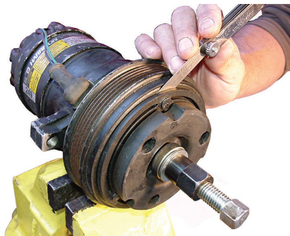
FIGURE 3-21 On some compressors, the air gap is adjusted by pressing the plate to the correct position.
