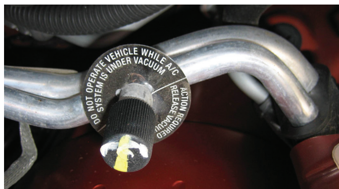
FIGURE 3-12 This tag on the service port indicates a damper-drive compressor that can be damaged if the engine is run without refrigerant in the system.
