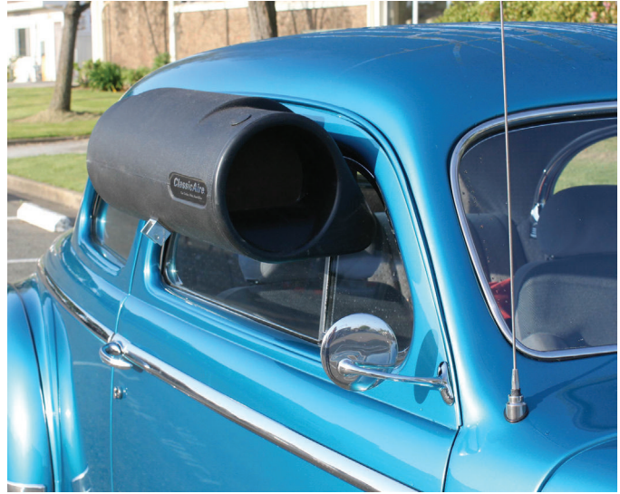
FIGURE 1-10 At one time, evaporative coolers were used to cool car interiors. Air forced through a water-wetted mesh produces evaporation and a cooling effect.
