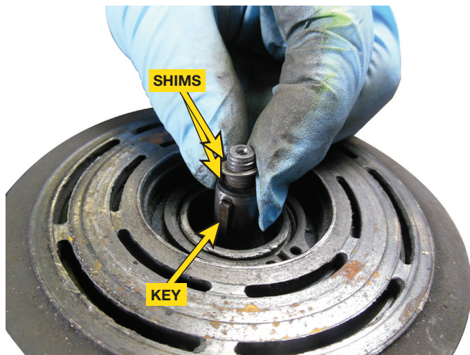
FIGURE 3-20 Air gap of the clutch is adjusted on some A/C compressors by using thin metal washers called shims. Adding a shim increases the gap and deleting a shim decreases the gap.
