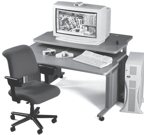
Figure 1.7 Intergraph Image Station Z softcopy plotter. (From Elements of Photogrammetry: With Applications in GIS , by Wolf and Dewitt, 2000, Courtesy Intergraph, Inc., and the McGraw- Hill Companies.)
