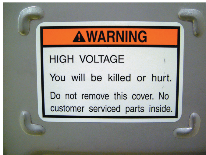
FIGURE 1-84 A warning label on a Honda hybrid warns that a person can be killed due to the high-voltage circuits under the cover.
