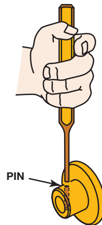
FIGURE 1-46 A punch used to drive pins from assembled components. This type of punch is also called a pin punch.
