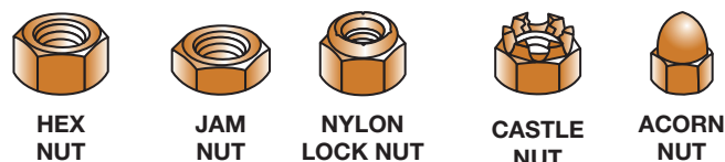
FIGURE 1-13 Nuts come in a variety of styles, including locking (prevailing torque) types, such as the distorted thread and nylon insert type.
