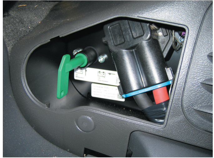
FIGURE 1-87 The shut-off switch on a GM parallel hybrid truck is green because this system uses 42 volts instead of higher, and possibly fatal, voltages used in other hybrid vehicles.
