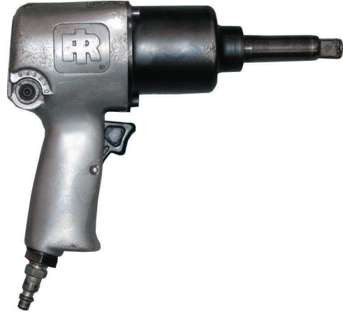
FIGURE 1-55 A typical 1/2 inch drive air impact wrench. The direction of rotation can be changed to loosen or tighten a fastener.
