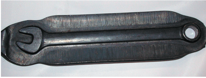
FIGURE 1-15 A wrench after it has been forged but before the flashing, extra material around the wrench, has been removed.
