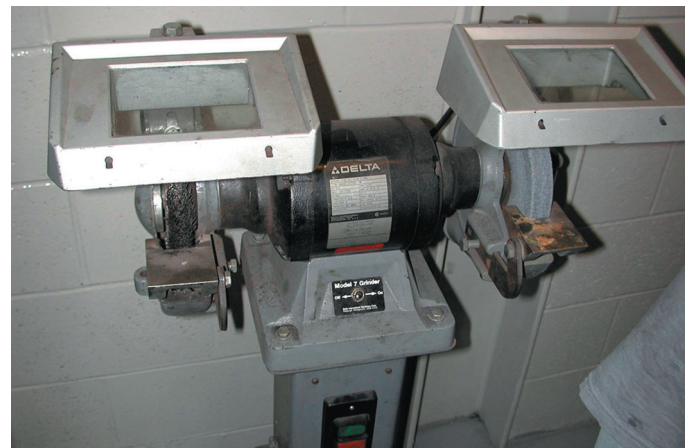
FIGURE 1-60 A typical pedestal grinder with a wire wheel on the left side and a stone wheel on the right side. Even though this machine is equipped with guards, safety glasses or a face shield should always be worn whenever using a grinder or wire wheel.
