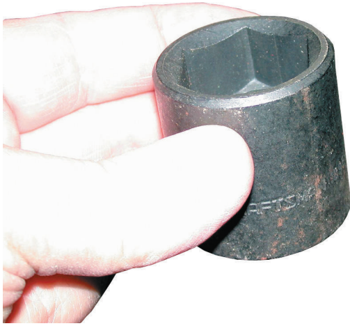
FIGURE 1-57 A black impact socket. Always use an impact-type socket whenever using an impact wrench to avoid the possibility of shattering the socket, which could cause personal injury. If a socket is chrome plated, it is not to be used with an impact wrench.
