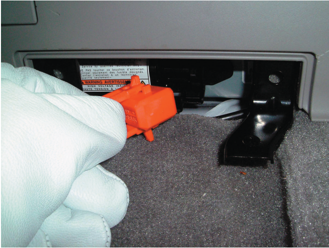
FIGURE 1-85 The high-voltage disconnect switch is in the trunk area on a Toyota Prius. Insulated rubber lineman's gloves should be worn when removing this plug.
