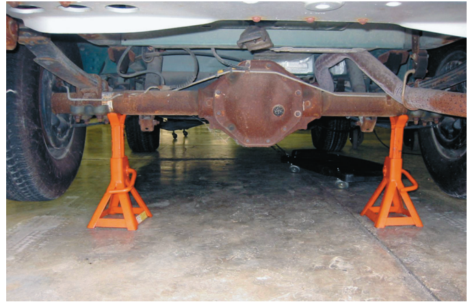
FIGURE 1-75 (a) A hydraulic hand-operated floor jack. (b) Whenever a vehicle is raised off the ground, a safety stand should be placed under the frame, axle, or body to support the weight of the vehicle.
