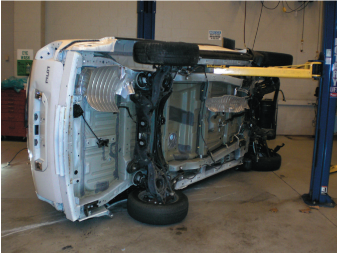
FIGURE 1-72 This training vehicle fell from the hoist because the pads were not set correctly. No one was hurt but the vehicle was damaged.
