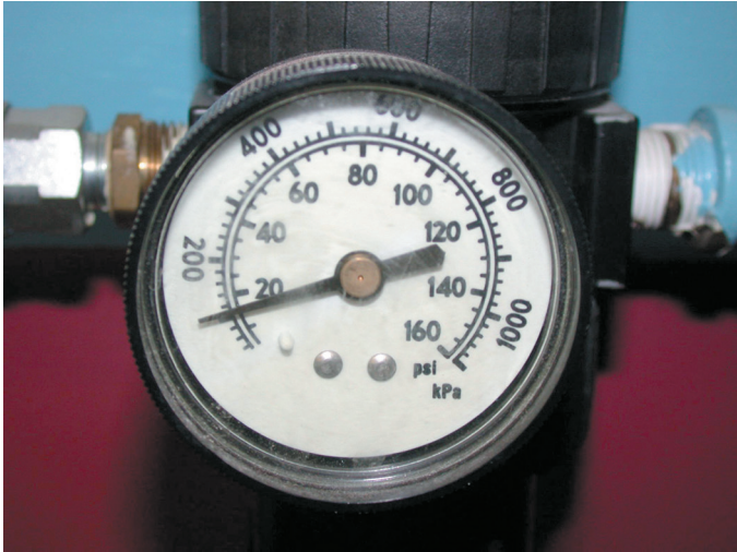
FIGURE 1-11 The air pressure going to the nozzle should be reduced to 30 PSI or less.
