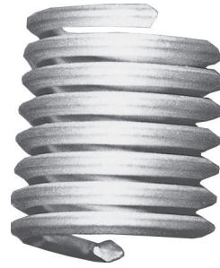
FIGURE 3-24 Helical inserts look like small, coiled springs. The outside is a thread to hold the coil in the hole, and the inside is threaded to fit the desired fastener.
