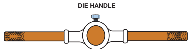
FIGURE 3-12 A die handle used to rotate a die while cutting threads on a metal rod.
