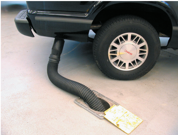
FIGURE 1-6 Always connect an exhaust hose to the tailpipe of the engine of a vehicle to be run inside a building.
