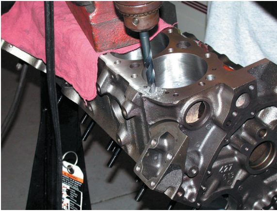
FIGURE 3-29 Drill out the damaged threads with the correct bit.
