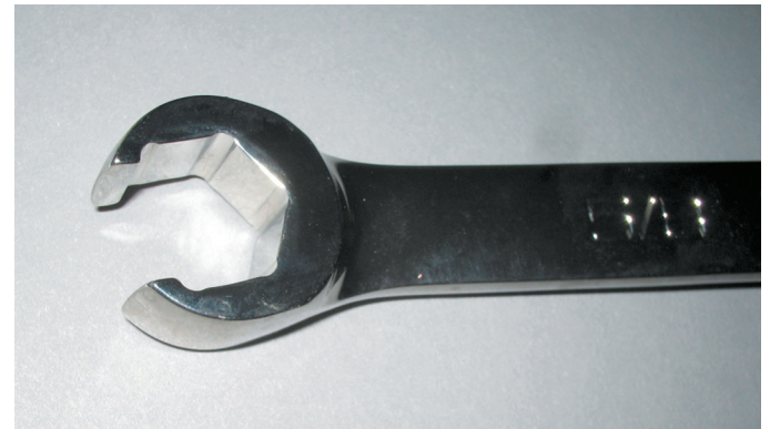
FIGURE 4-7 The end of a typical line wrench, which shows that it is capable of grasping most of the head of the fitting.
