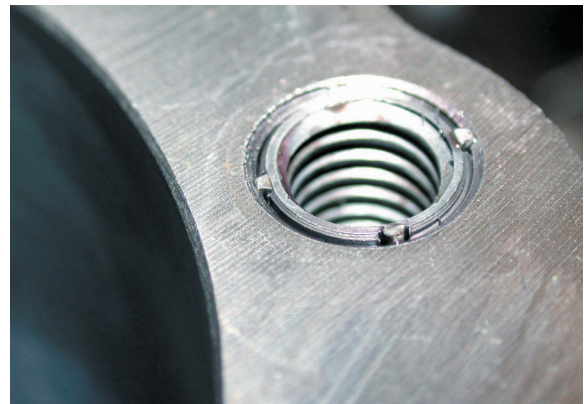
FIGURE 3-33 The insert and insert locks should be below the surface of the workpiece.
