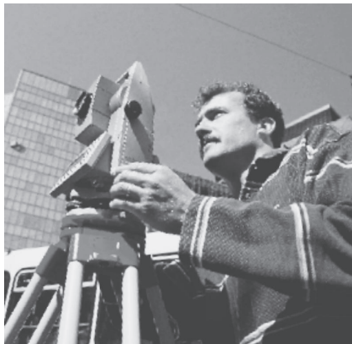
Figure 1.4 LEICA TPS 1100 total station instrument. (Courtesy Leica Geosystems, Inc.)
