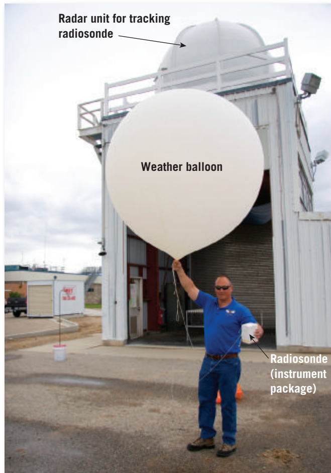
▲ Figure 1.21 Radiosonde This lightweight package of instruments is carried aloft by a small weather balloon. It transmits data on vertical changes in temperature, pressure, and humidity in the troposphere. The troposphere is where practically all weather phenomena occur, so it is very important to have frequent measurements.
