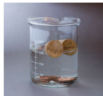
▲ Figure 1.9 At room temperature, the density of water is approximately 1.00 g/mL. A coin sinks in water, but a cork floats on water.
