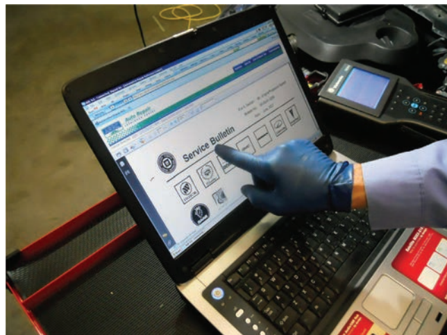
FIGURE 1-9 After checking for stored diagnostic trouble codes (DTCs), the wise technician checks service information for any technical service bulletins that may relate to the vehicle being serviced.
