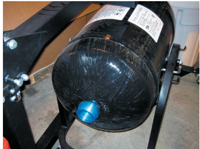
FIGURE 2-28 A CNG storage tank from a Honda Civic GX shown with the fixture used to support it while it is being removed or installed in the vehicle. Honda specifies that three technicians be used to remove or install the tank through the rear door of the vehicle due to the size and weight of the tank.
