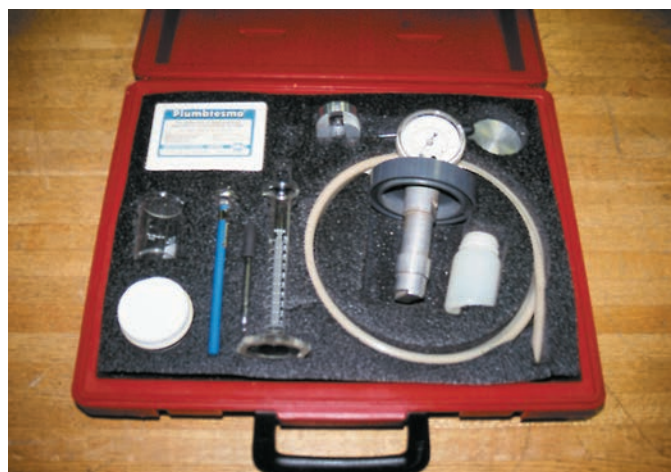
FIGURE 2-3 A gasoline testing kit, including an insulated container where water at 100°F is used to heat a container holding a small sample of gasoline. The reading on the pressure gauge is the Reid vapor pressure (RVP).
