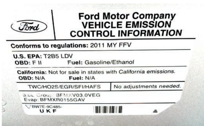
FIGURE 2-23 This flexible fuel vehicle (FFV) vehicle emission control information (VECI) sticker located under the hood indicates that it can operate on either gasoline or ethanol.
