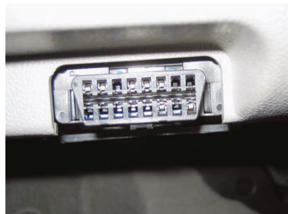
FIGURE 1-17 A typical OBD-II data link connector (DLC). The location varies with make and model and may even be covered, but a tool is not needed to gain access. Check service information for the exact location if needed.
