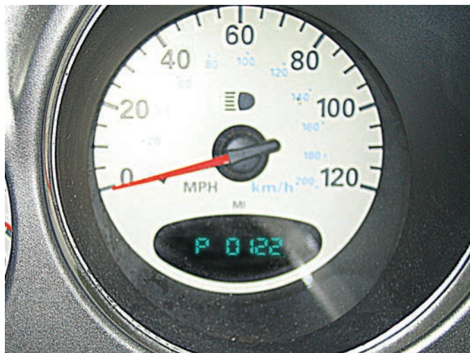
FIGURE 1-15 Diagnostic trouble codes (DTCs) from Chrysler and Dodge vehicles can be retrieved by turning the ignition switch to on and then off three times.
