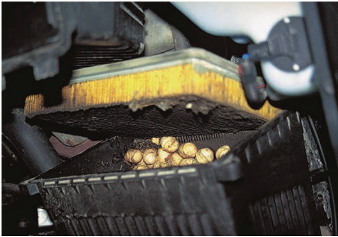
FIGURE 1-5 This is what was found when removing an air filter from a vehicle that had a lack-of-power concern. Obviously the nuts were deposited by squirrels or some other animal, blocking a lot of the airflow into the engine.
