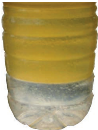
FIGURE 2-11 A container with gasoline containing water and alcohol. Notice the separation line where the alcohol-water mixture separated from the gasoline and sank to the bottom.
