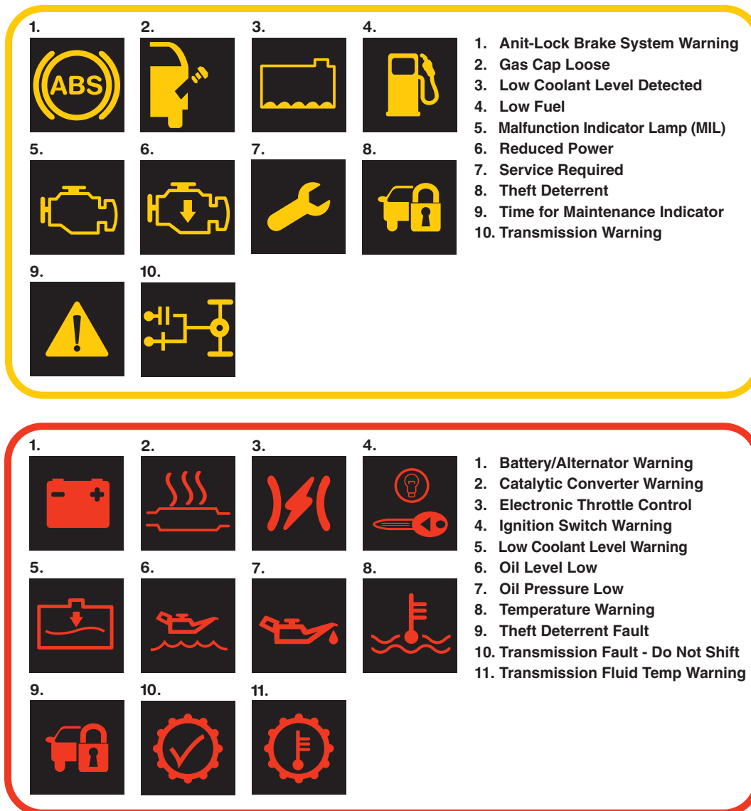
FIGURE 1-3 The amber dash warning symbols indicate that a fault has been detected. A red dash warning light indicates that a major fault has been detected requiring action by the driver as soon as possible.
