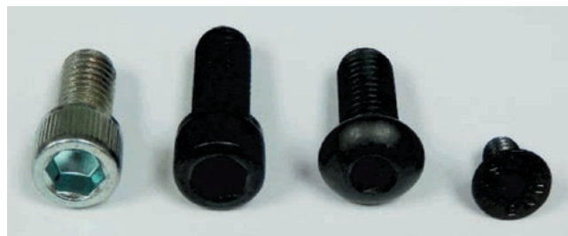
Figure A-17 Various cap screws. From the left: a stainless-steel socket-head cap screw, a regular socket-head cap screw, a button-head cap screw, and a flat-head cap screw (Courtesy of Fox Valley Technical College).
