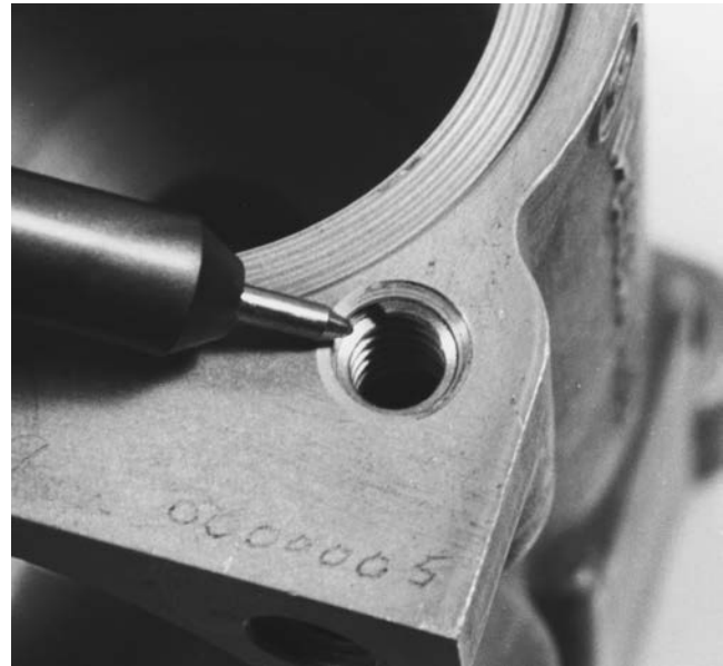
Figure A-23 Stainless steel thread insert used in an aluminum valve housing.
