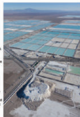
▲ Figure 4.4.2 Lithium Processing in San Pedro de Atacama, Chile In the high Andes, lithium-rich brine is pumped out of the ground and into evaporation ponds. Once dried, the powdery substance is shipped and processed into lithium.
