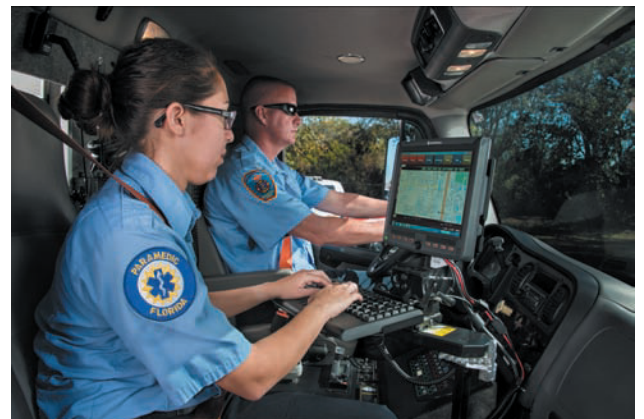
Figure 1.4 A typical device with GPS capability installed in an emergency vehicle.
