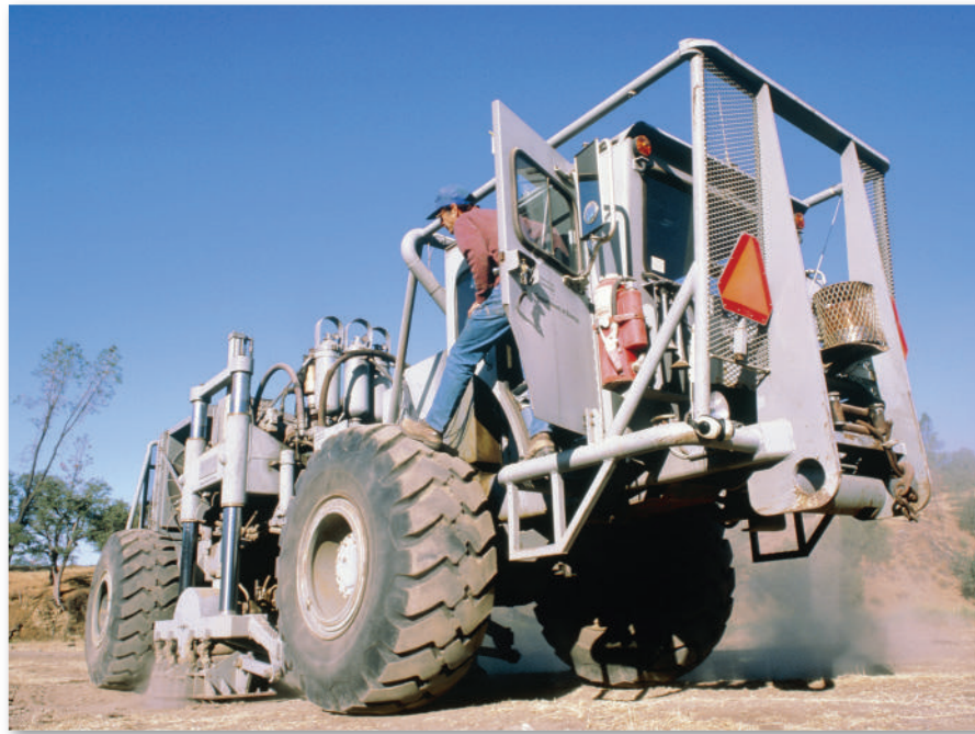
◀ Figure 1.9 Observation and measurement Scientific data are gathered in many ways. This piece of equipment produces artificial earthquake waves, which are used to probe the underlying rock structures. Vibrations from the 26-ton truck are transmitted to the ground by way of a baseplate (visible between the wheels). The waves reflect from rock layers and structures and are recorded by a network of seismographs.
