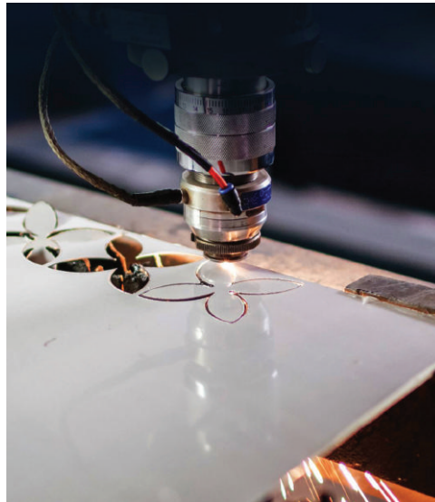
Figure I.8: Cutting sheet metal with a laser beam. Source: Courtesy of SPI Lasers UK Ltd.
