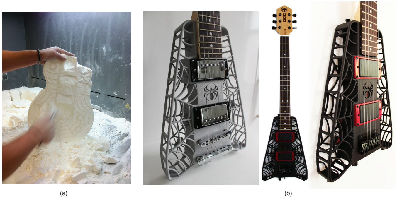
Figure I.5: Guitars produced through additive manufacturing. (a) Spider design being removed from a powder bed. Note that the support material, or cake , has some strength and needs to be carefully removed. (b) Finished Spider guitars. Source: Courtesy of O. Diegel.
