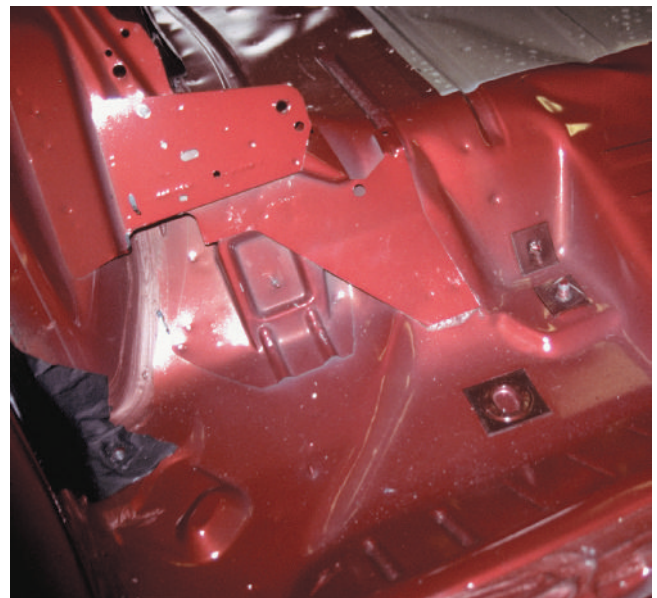
FIGURE 1-5 Note the ribbing and the many different pieces of sheet metal used in the construction of this body.
