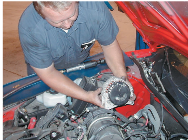
FIGURE 1-10 The alternator is responsible for supplying the electrical needs of the vehicle and to keep the battery charged.
