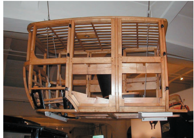
FIGURE 1-2 Most vehicle bodies were constructed with a wood framework until the 1920s.
