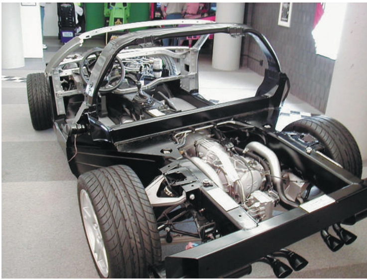
FIGURE 1-6 A Corvette without the body. Notice that the vehicle is complete enough to be driven. This photo was taken at the Corvette Museum in Bowling Green, Kentucky.
