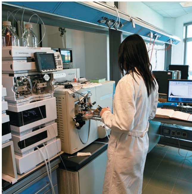
A Scientist Preparing an Injection for Mass Spectrometry.
