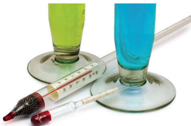
FIGURE 1.6 Hydrometers are carefully calibrated and then placed in fluid to accurately measure fluid density. (Source: YAUHENI MESHCHARAKOU/123RF and Ellirra/123RF).
