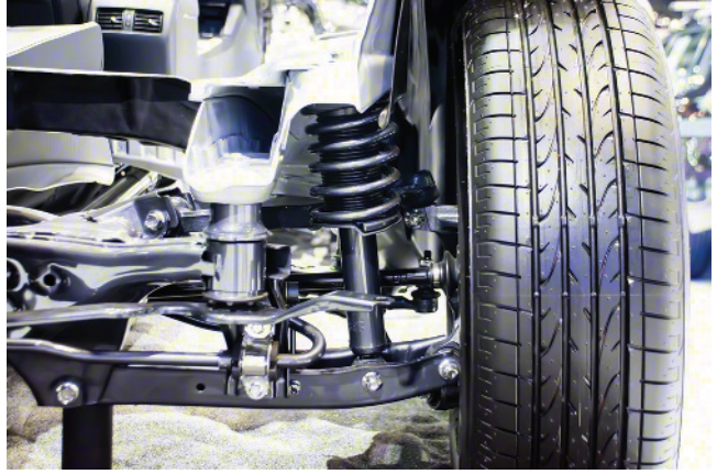
Figure 1.8 Close up of a vehicle suspension system showing the spring mechanism. (Photo courtesy of ScofieldZa/Shutterstock.)
