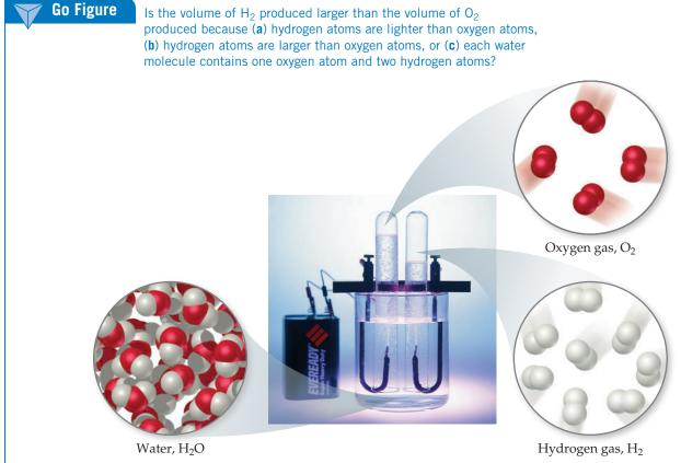
▲ Figure 1.6 Electrolysis of water. Water decomposes into its component elements, hydrogen and oxygen, when an electrical current is passed through it. The volume of hydrogen, collected in the right test tube, is twice the volume of oxygen.
