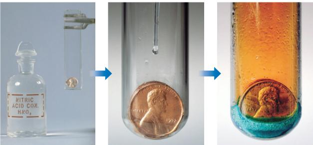
▲ Figure 1.10 The chemical reaction between a copper penny and nitric acid. The dissolved copper produces the blue-green solution; the reddish-brown gas produced is nitrogen dioxide.
