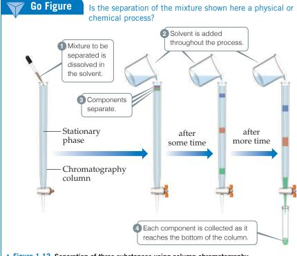
▲ Figure 1.13 Separation of three substances using column chromatography.
