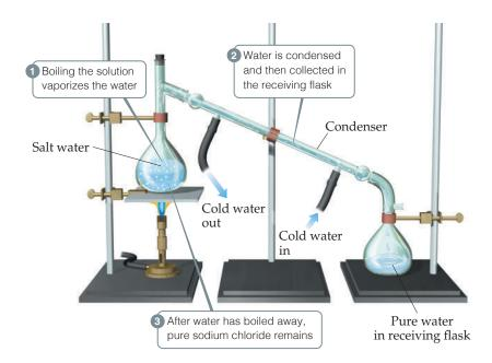
An important method of separating the components of a homogeneous mixture is **distillation**, a process that depends on the different abilities of substances to form gases. For example, if we boil a solution of salt and water, the water evaporates, forming a gas, and the salt is left behind. The gaseous water can be converted back to a liquid on the walls of a condenser, as shown in **Figure 1.12**.
