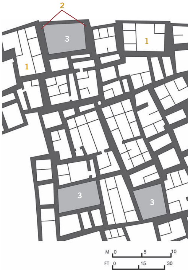
Figure 1.1-10 Çatalhöyük, southern Turkey. Plan of a district of the city, seventh millennium BCE, showing (1) individual cellular units with platforms and internal parapets, (2) party walls connecting individual units (there were no doors in these walls; inhabitants entered through the roofs), and (3) courtyards between units.
