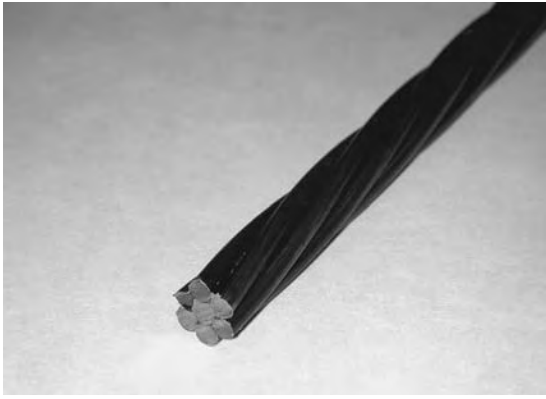
Figure 1.13.4 Typical 7-wire strand used in prestressed concrete construction (Photo by José A. Pincheira.)
