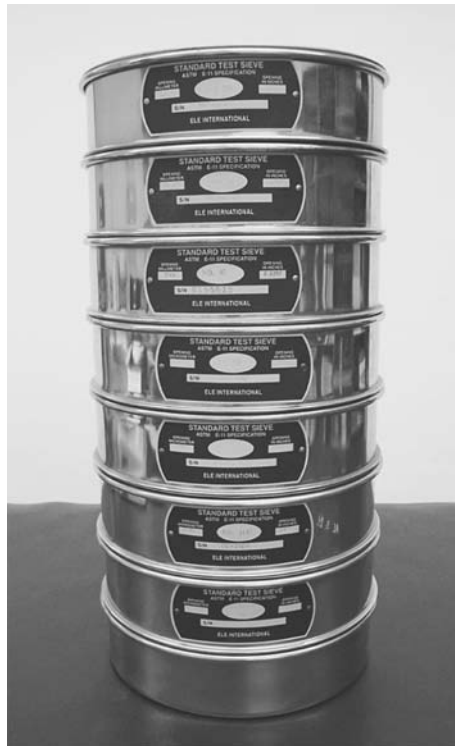
Figure 4-1. Stack of sieves with a pan at the bottom and a cover at the top.
