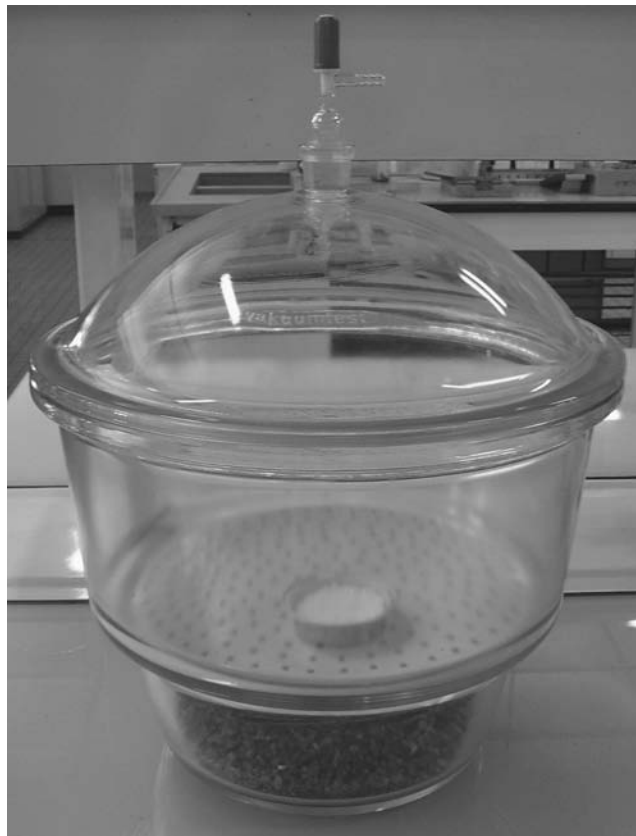
Figure 2-2. A desiccator. [Courtesy of N. Sivakugan, James Cook University, Australia.]
