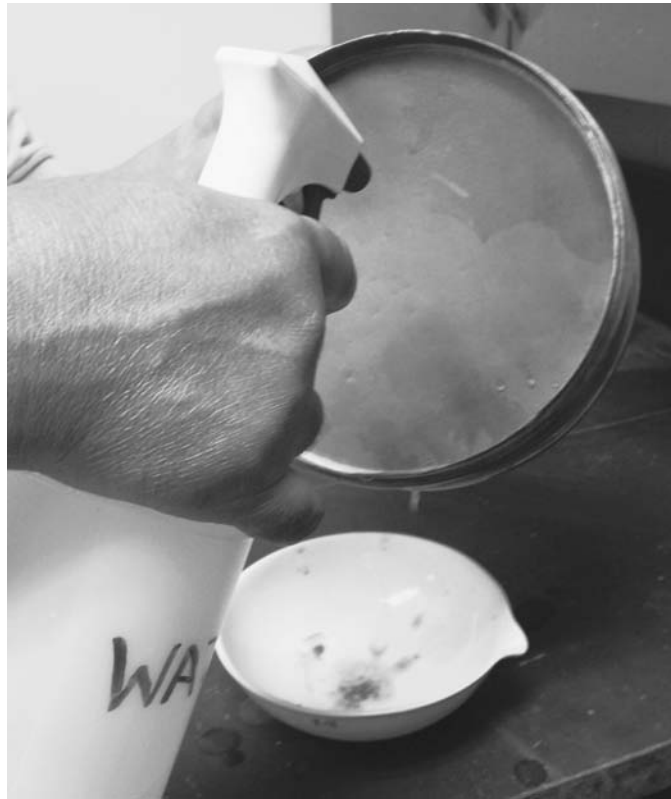
Figure 4-4. Back washing to transfer soil retained on No. 200 sieve to an evaporating dish.
