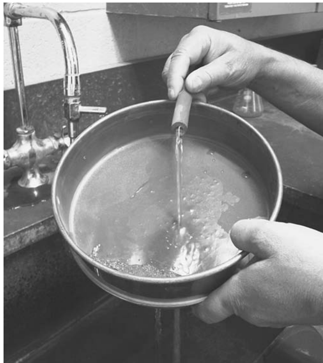
Figure 4-3. Washing of soil retained on No. 200 sieve.
