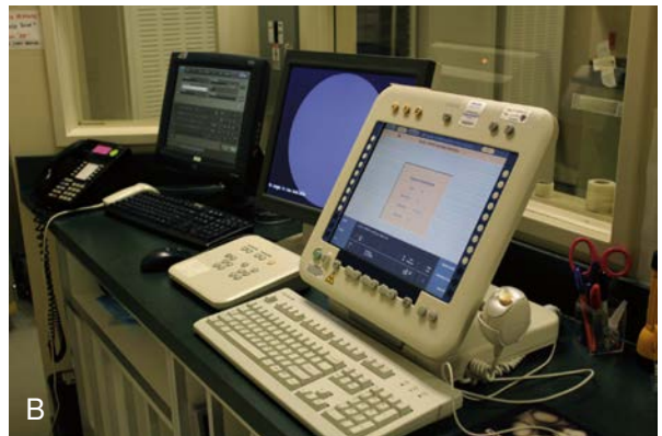
Fig. 1.26 Examples of x-ray control consoles. (A) Simple computerized radiographic controls. (B) Controls for filmless radiography with digital fluoroscopy.
