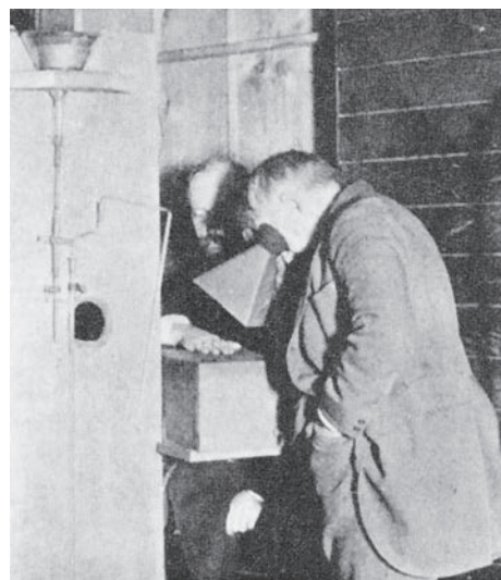
FIGURE 1.8 Thomas Edison is seen viewing the hand of his unfortunate assistant, Clarence Dally, through a fluoroscope of his own design. Dally's hand rests on the box that contains the x-ray tube.
