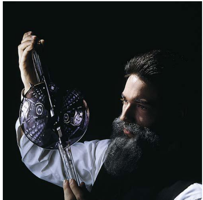
FIGURE 1.5 The type of Crookes tube Roentgen used when he discovered x-rays. Cathode rays (electrons) leaving the cathode are attracted by high voltage to the anode, where they produce x-rays and fluorescent light. (Courtesy Gary Leach, Memorial Hermann Hospital.)
