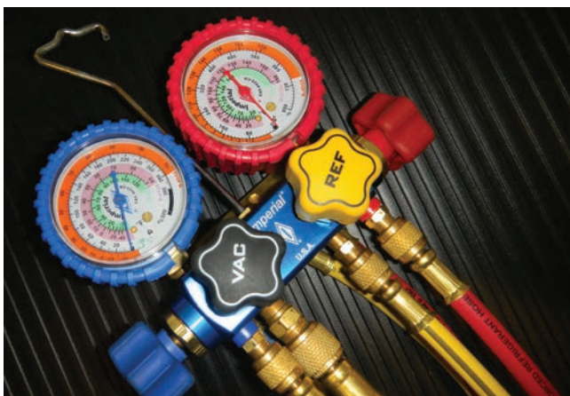
Figure 1.2 Pressure gauge used to measure operating pressures in air-conditioning and refrigeration equipment. Photo by Eugene Silberstein
