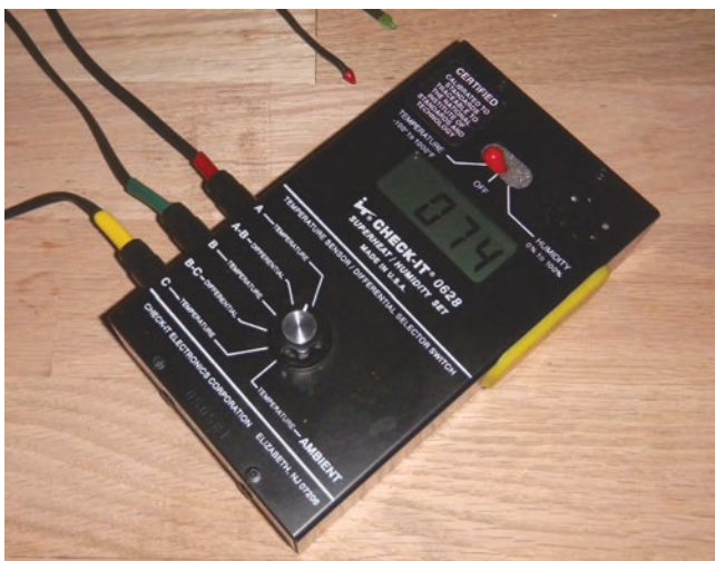
Figure 1.1 Thermocouple thermometer used to take accurate temperature readings in heating, air-conditioning, and refrigeration systems. Photo by Eugene Silberstein
