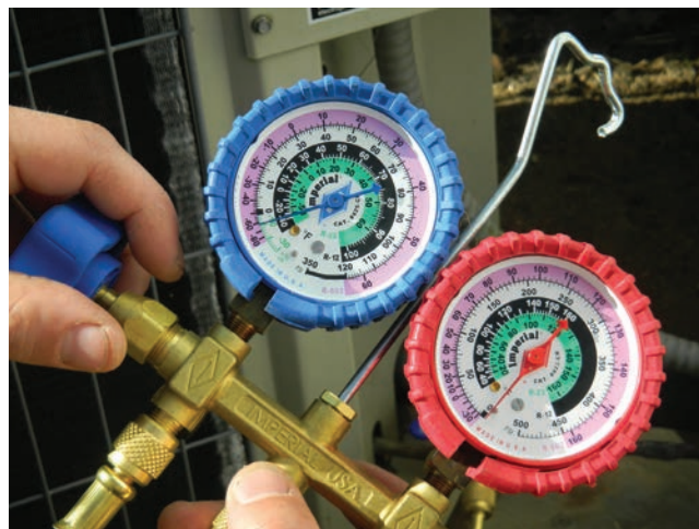
Figure 1.22 The gauge on the left, called a compound gauge , reads pressures above and below atmospheric pressure. The gauge on the right, called the high-pressure (high-side) gauge , will read up to 500 psi. Photo by Eugene Silberstein
