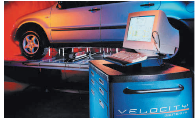
A To use this modern computerized measuring system, targets are hung from specific points on a vehicle. Laser light is reflected off the targets to make quick, accurate readings of the distance between targets.
