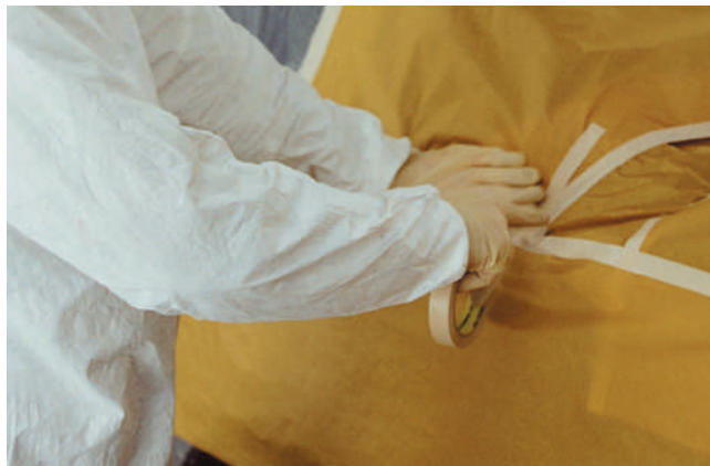
A Here a technician uses masking tape and masking paper to cover the area not to be painted.
