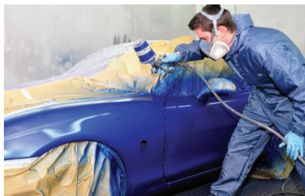
FIGURE 1-29 Excellent hand-eye coordination and specialized knowledge is needed to be a professional painter. (A) When painting a vehicle, keep the gun the correct distance from the surface. Also keep the gun parallel with the surface. (B) When painting, try to move the spray gun smoothly and evenly. Use straight line paint strokes that overlap evenly. If you move the gun at different speeds or move it further or closer to the surface, paint problems will result.
