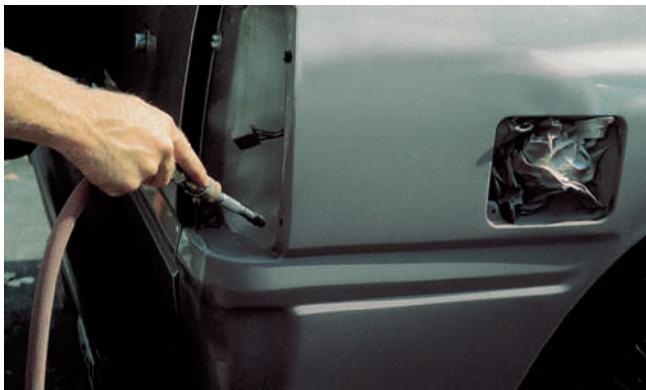
FIGURE 1-20 Before masking and priming, use a blowgun to clean the vehicle of dust and debris. Aim the blowgun down into all gaps between parts that could hold dust and dirt. Do this before final masking and moving the vehicle into the paint booth.
