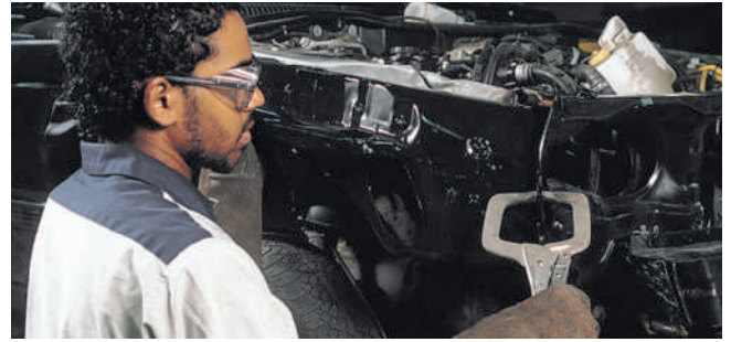
A New structural parts must be temporarily held in place with clamping pliers or screws.
