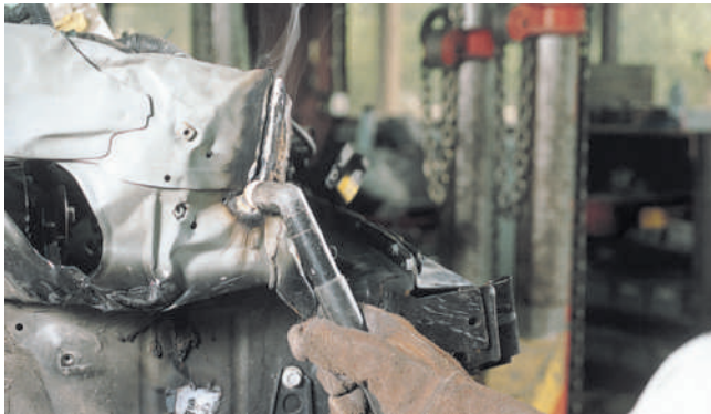
A Here a technician uses a plasma arc cutter to slice off a part for replacement.
