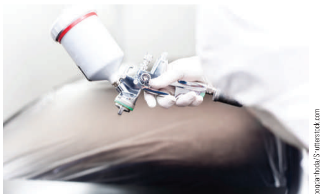
FIGURE 1-28 The spray gun is the main tool of a refinish technician. It must be adjusted properly to produce a smooth, even paint film on the vehicle.
