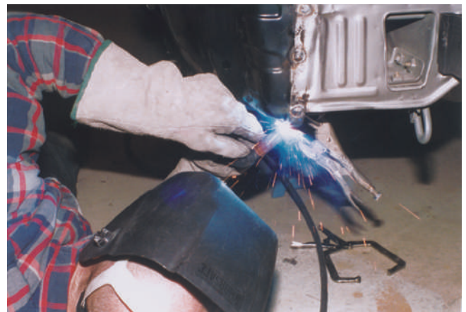
FIGURE 2-18 This technician is wearing a welding-type cartridge respirator and an automatic dimming welding helmet while making plug welds during panel replacement. Both are needed for protection when arc welding today's steel and aluminum panels during structural body repair.
