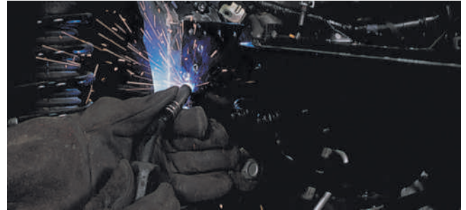
B First, tack weld parts in place, using only a few welds to hold the parts in alignment.
