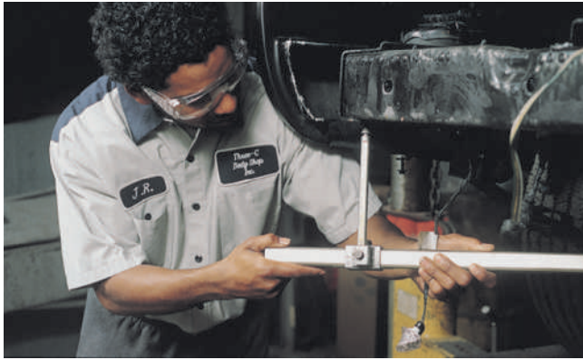
FIGURE 1-12 Constantly measure as you pull out damage. This will let you pull in the right direction with the right amount of power. Here the tram gauge has been set to vehicle specs and compared to reference points on the damaged vehicle. If the tram gauge does not align with reference points on the vehicle, further pulling is needed until the points are lined up to specifications.
