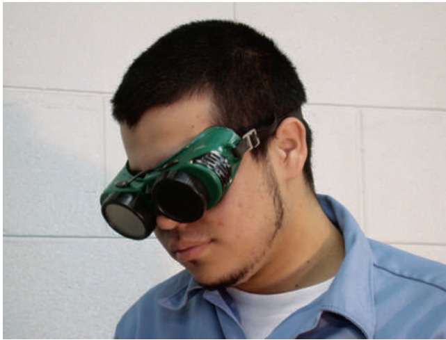
FIGURE 2-16 These tinted goggles should be worn when flame heating and torch cutting. Their shaded lens is dark enough for the brightness of a welding flame, but not dark enough to protect your eyes when electric welding.
