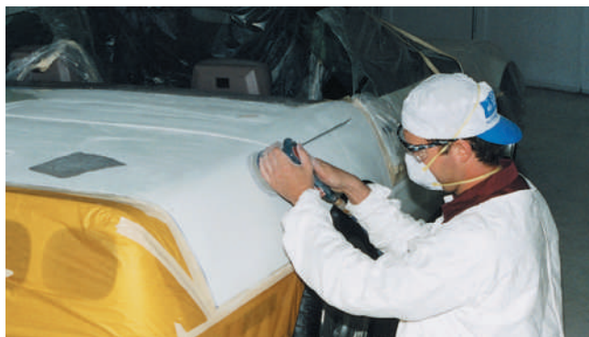
B An orbital sander or hand sanding with a block and fine sandpaper is needed to scuff the old paint to prepare it to accept and bond with the new paint.
