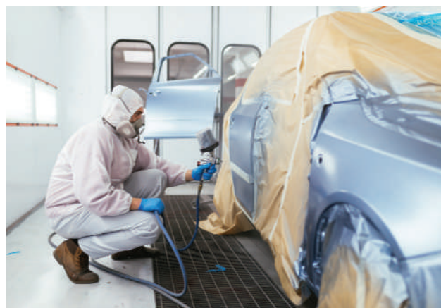
FIGURE 1-30 Here a refinish technician is spraying the colorcoat along the bottom and side of the car body. This will be followed by spraying the clearcoat to bring out the gloss or shine.
