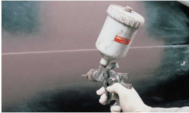
FIGURE 1-22 Self-etch or epoxy primer must be sprayed over all bare metal to bond to the metal. Primer-surfacer is often sprayed over body filler and the repair area to help level the repair area. Allow each coat of primer to flash properly before applying the next coat.
