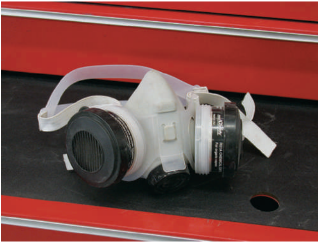
FIGURE 2-7 A cartridge-type respirator will filter fine particles, mists, and some fumes that a dust respirator will not stop.
