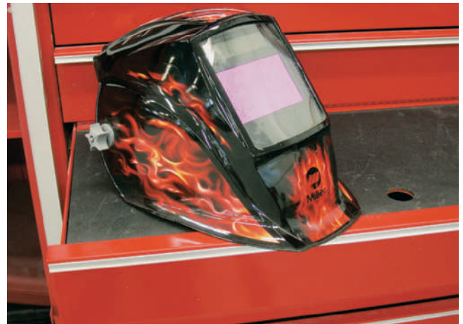
A This welding helmet has a self-darkening lens. It is only lightly shaded until you start welding and then it darkens enough to protect your eyes.
