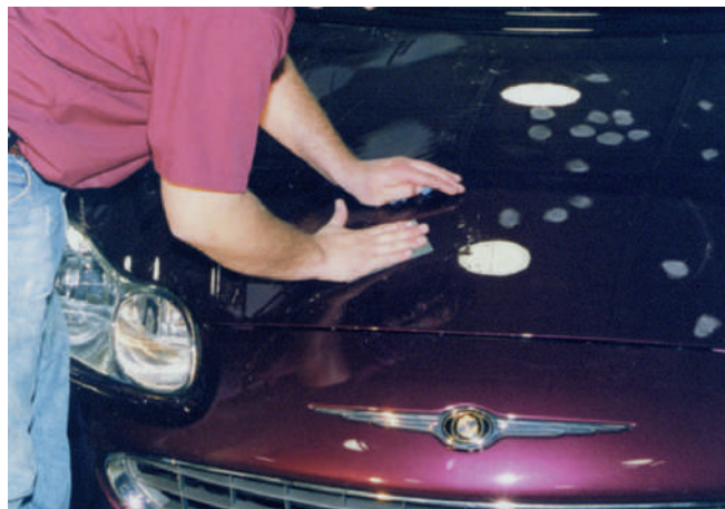
A After paint cures properly overnight, it may be necessary to wet sand out any imperfections, such as a small dirt nib or adjust the orange peel. Use a small sanding block and ultrafine (1000 or finer grit) sandpaper, and be careful not to cut through the clearcoat, or repainting will be required.
