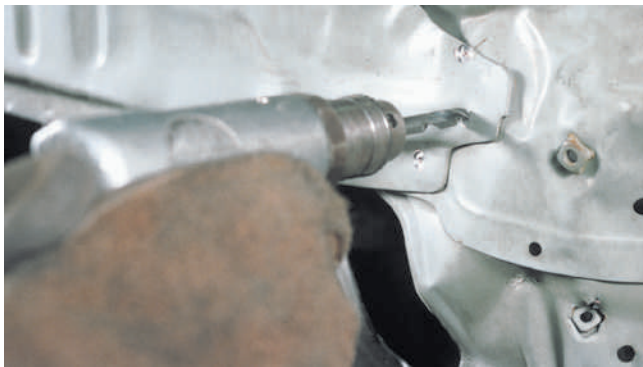
B Many parts or panels are attached with spot welds. A spot weld remover, a specialized drill, is often used to cut out each spot weld for part removal.
