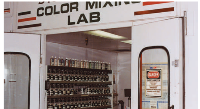
FIGURE 1-25 Most large body shops have their own paint mixing room. It has all color pigments and other ingredients for mixing paint materials. Mixing rooms also have forced ventilation to prevent buildup of paint fumes.
