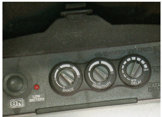
B Controls on the inside of the self-darkening helmet allow you to adjust how fast and dark the lens gets when you are welding.
