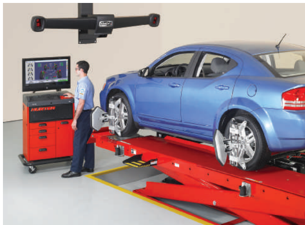
A A technician uses special equipment to adjust wheel alignment. This must be done if suspension parts are damaged in an accident.
