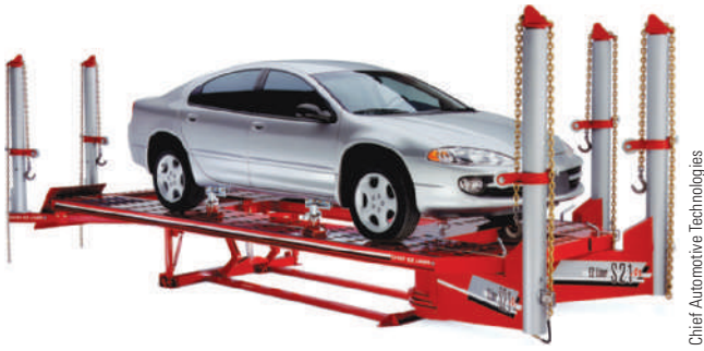
FIGURE 1-10 A frame rack is a heavy steel framework with hydraulic equipment for forcing major structural parts back into alignment. The vehicle is anchored to the rack so it cannot move. Then pulling towers and chains can be attached to the damaged section of the vehicle to pull out the structural damage.
