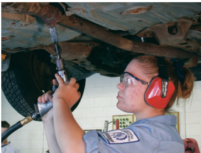
FIGURE 2-21 Many shop tools produce very high decibel levels. This air chisel being used to remove a badly rusted exhaust system is a good example. Its sound level is loud enough to cause permanent hearing loss.
