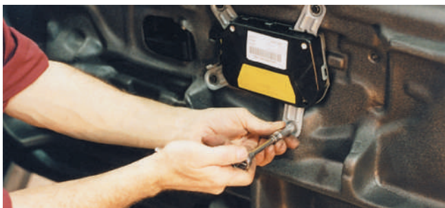
FIGURE 1–17 A technician replaces a small air bag located on the inside of the door frame. Note how the technician stays to one side in case the air bag accidentally deploys. Air bags deploy with a “bang” and can cause injury to your arms, hands, and face.
