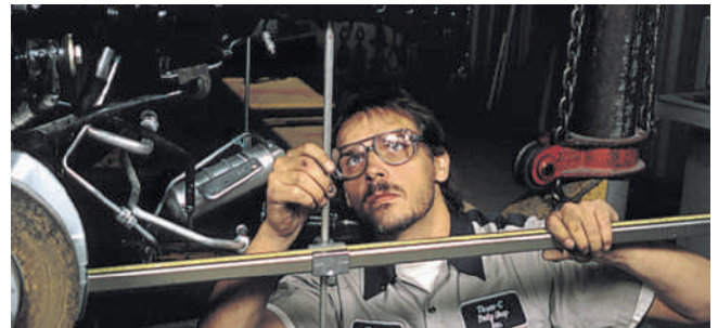
C After tack welding a part, measure its location before final welding. You may need to adjust a part's position while it is still tacked in place.
