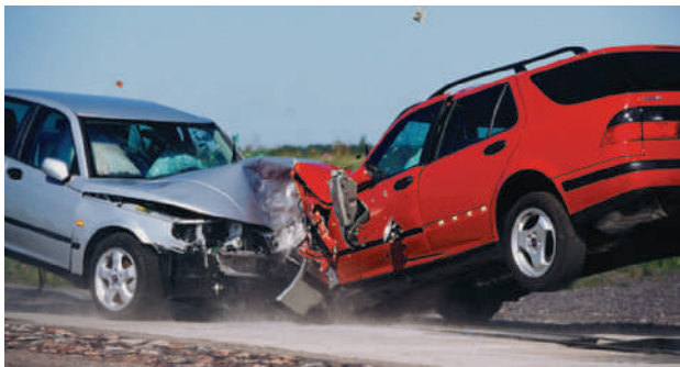
FIGURE 1-1 During a major collision, like this head-on crash test, tremendous energy is dissipated into the body/frame structures of both cars. Modern vehicles are designed to absorb this energy by controlled collapse of structural body/frame members. The front and rear ends of the vehicles are designed to crush or collapse while keeping the passenger compartment intact. With today’s front and side air bags and seat belts, the drivers and passengers would suffer little or no injury in this violent collision.
