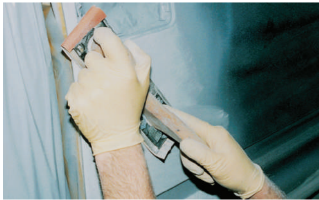
A A large sanding block is commonly used to smooth and level the repair area with the surrounding undamaged areas.
