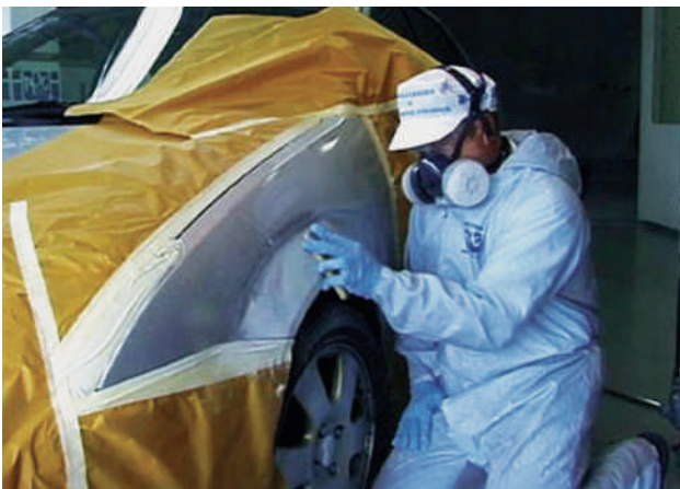
FIGURE 2-8 Cartridge-type respiratory masks will filter finer particles than fiber dust masks. They provide adequate protection from most primers, sealers, and noncatalyzed paints.
