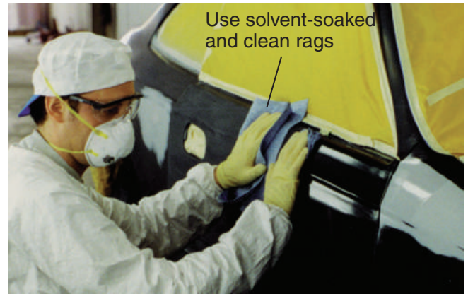
FIGURE 1-24 Before painting, use two lint-free shop towels to wipe the repair area clean. First, use a shop towel soaked with wax and grease remover to remove any surface contaminants. Then use a clean shop towel to wipe the surface while the solvent is still wet.
