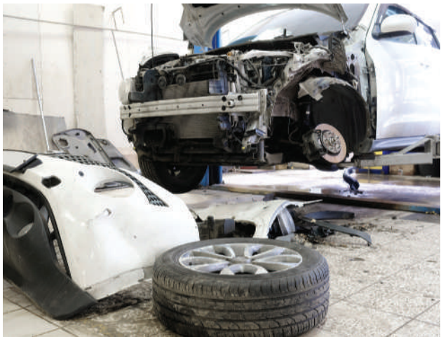
FIGURE 1-8 To start work, you must normally remove damaged outer body parts to gain access to hidden parts that require straightening or replacement. Here the technician is removing a front fender.
