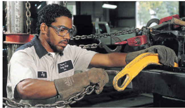
B After the vehicle is anchored, pulling clamps and chains are attached to the area to be straightened.
