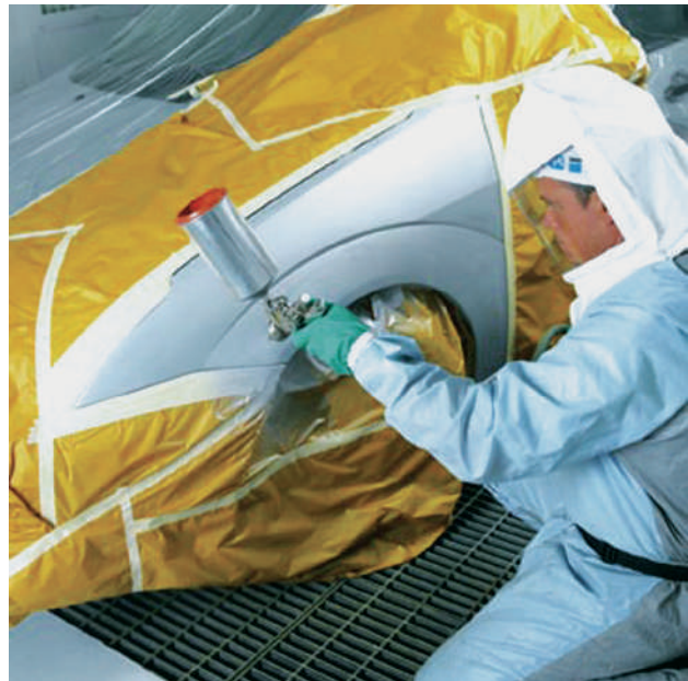
FIGURE 2-9 This refinish technician is wearing a state-of-the-art, air-supplied respirator while painting a car. It uses a lightweight hood with a clear lens. The hood keeps the head clean and also allows circulation of fresh breathing air.
