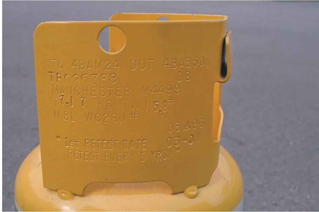
Figure 1-20 Service cylinders must be reinspected every 5 years.
