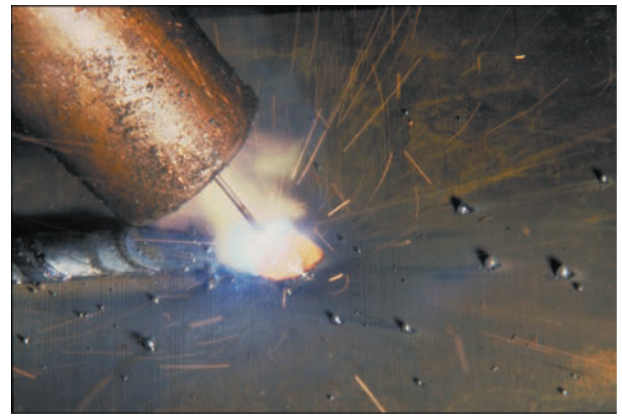
FIGURE 1-13 This GMA welding can be seen in the Gas Metal Arc Welding video series on tape 2.
