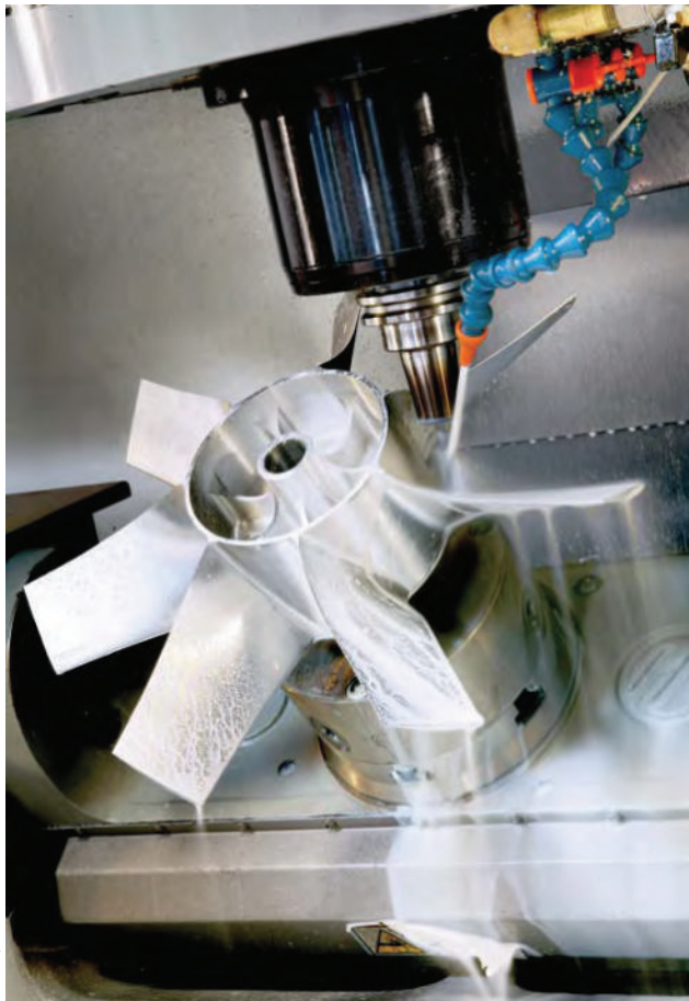
FIGURE 1.1.5 Today's state-of-the-art CNC machine tools can be programmed to run unattended and machine extremely complex shapes.
