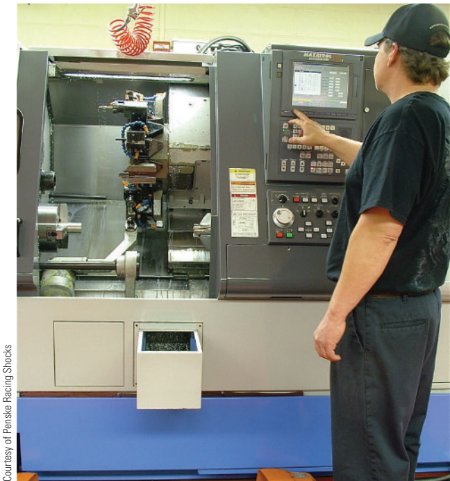
FIGURE 1.2.2 This set-up technician is setting up the cutting tools on a CNC lathe.
