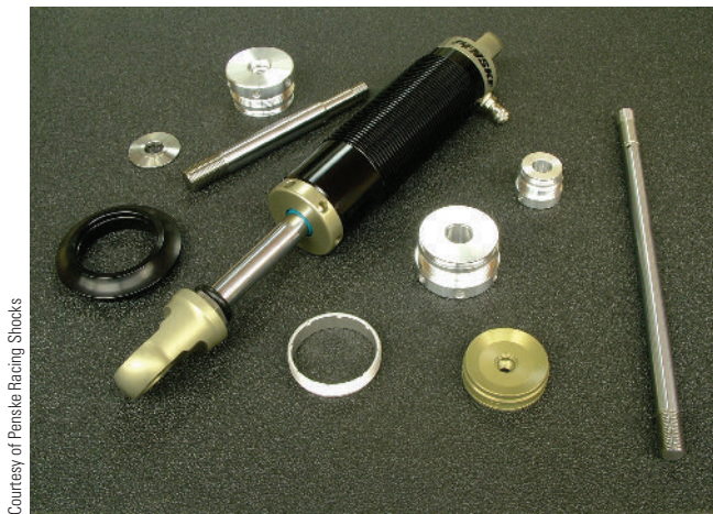
FIGURE 1.1.6 Machined shock absorber components and an assembled shock absorber used in motorsports racing.
