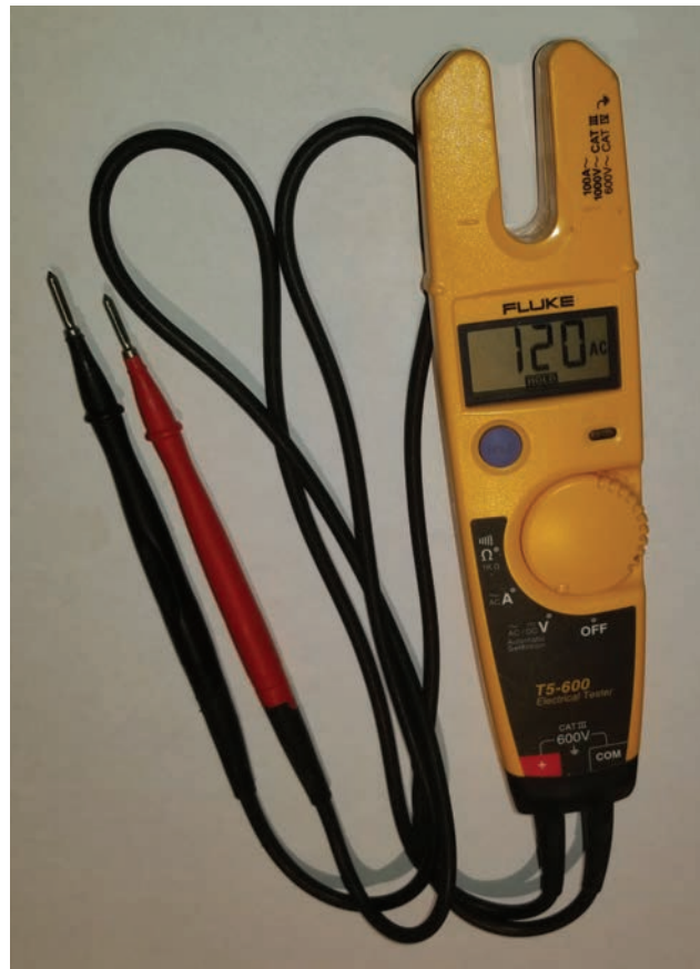
FIGURE 1-5 This digital volt-meter and amp-meter is rated Category III for voltage readings (contact through test leads) and Category IV for current readings (non-contact through open jaws).
