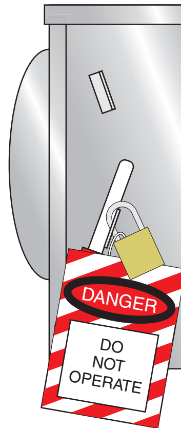
FIGURE 1-2 A typical disconnect switch with a lock and a tag attached to it. In the OSHA, ANSI, and NFPA standards, this is referred to as the lockout/tagout procedure.
