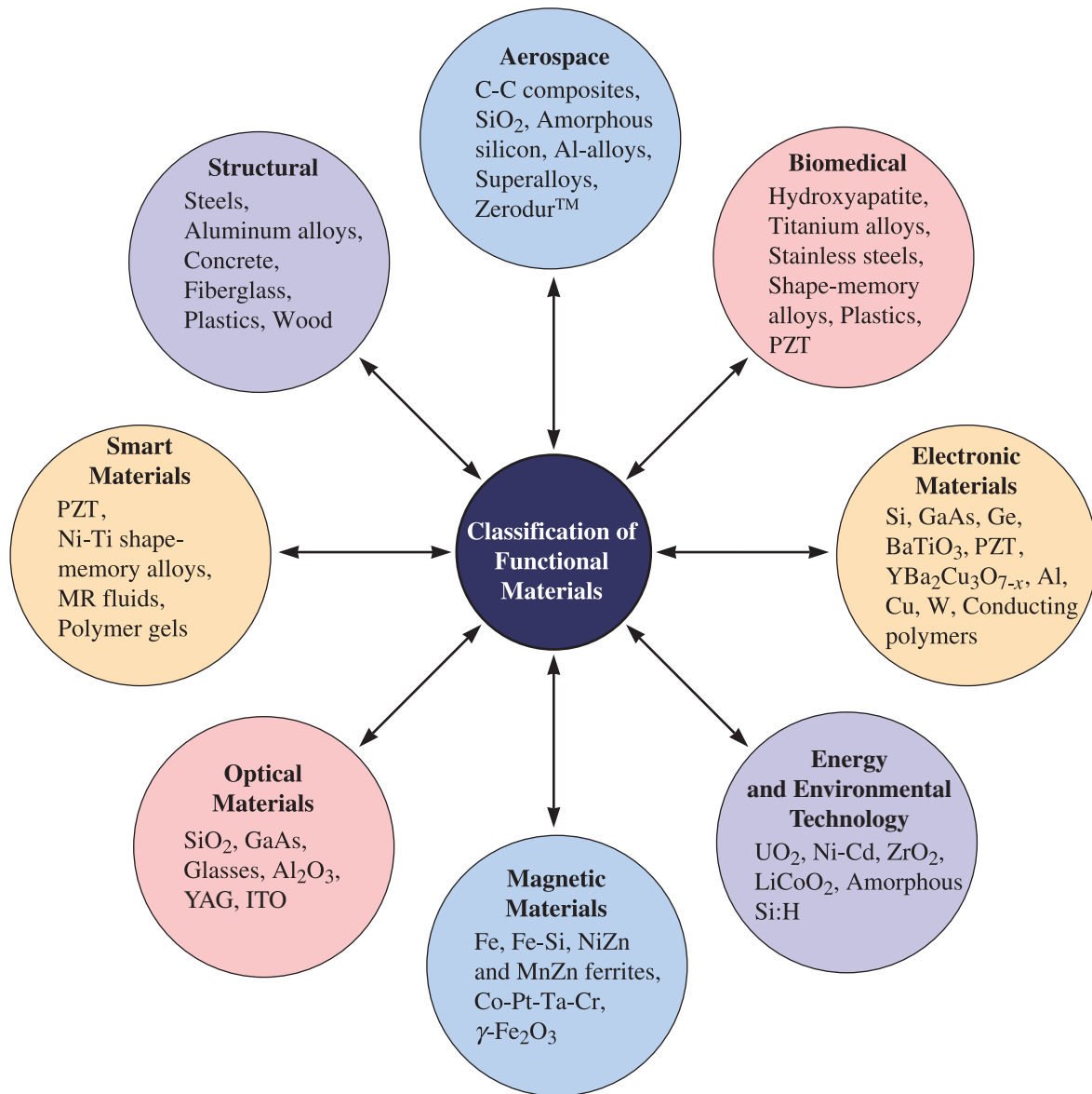
Figure 1-5 Functional classification of materials. Notice that metals, plastics, and ceramics occur in different categories. A limited number of examples in each category are provided.
