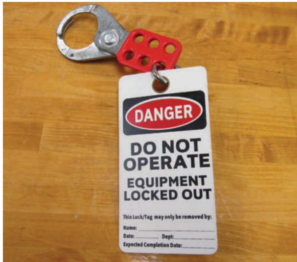
FIGURE 1-3 Tag used for the tag-out procedure.
