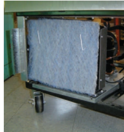
Fiberglass air filter on reach-in condenser
