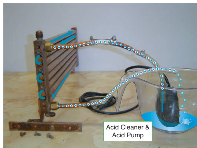
FIGURE 3-16 Acid cleaning illustration on a water-cooled condenser. Photo by Dick Wirz.
