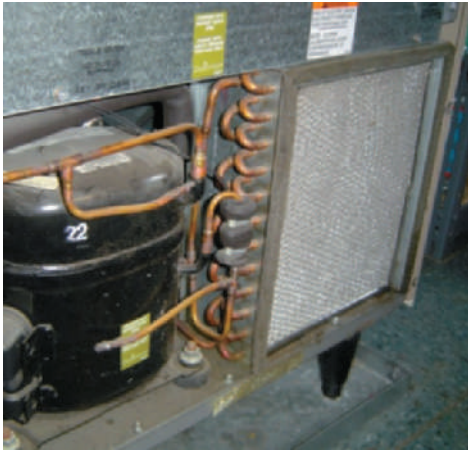
Metal mesh condenser air filter on ice machine
