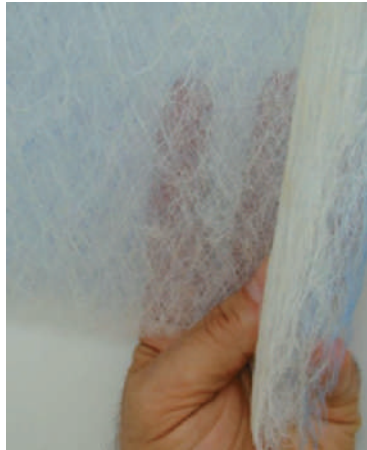
1" fiberglass material allows good airflow
