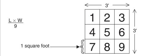
To calculate square yards, divide the area (square feet) by 9. There are 9 square feet in 1 square yard. It is highly recommended you always write the formula down before you begin to solve the equation. Write the formula down first, and carefully insert each number from the question into the formula.
