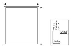
What is square footage of the 4-inch slab if the building dimension is 31 feet 6 inches  $\times$  20 feet?
