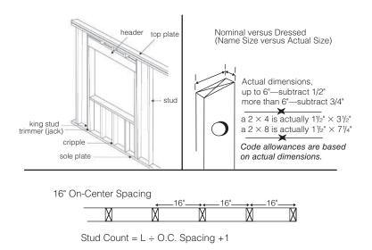
**Bottom (sole) plate** The bottom horizontal structural member of a stud-framed wall. The bottom plate is fastened to the floor (foundation or subfloor) with foundation bolts or proper nails.
