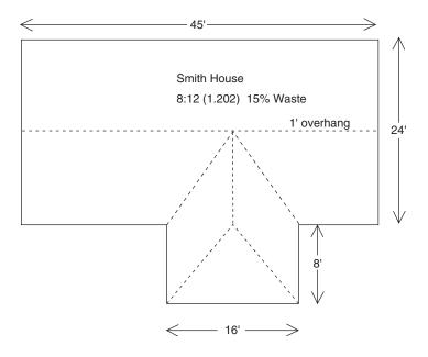
Now, one that is a little more difficult (Smith House on page 42). The building in the diagram provides all of the information necessary for calculating the area of the roof. It provides the roof slope as well as the roof multiplier. The waste factor for this plan is indicated, and the overhang is noted. Follow these steps:
