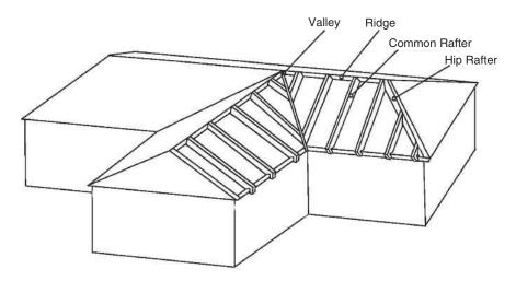
**Ridgeboard** The highest horizontal roof member, which serves to align the rafters and tie them together at the upper end. The ridgeboard is at least one size larger than the rafters. For example, if  $2 \times 8$ , one size larger is  $2 \times 10$ .
