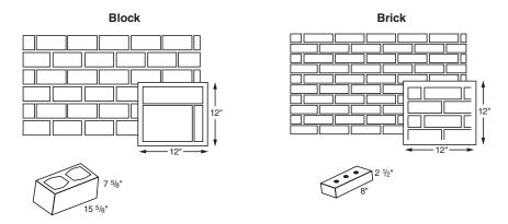
Estimating brick and block is similar to estimating gypsum or sheathing. Begin by determining the face area of the material to be installed. For example, if an  $8" \times 16"$  nominal block ( $75\%" \times 155\%"$  plus the mortar joint) is to be used, the face area of the block is 128 square inches. To convert this to a multiplier, you can follow one of several methods.
