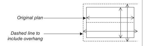
Let's try a simple roof. Calculate the roof area of a building that is  $30^{\circ}$  wide,  $45^{\circ}$  long, with a roof slope of 5:12. The overhang for the building is  $1^{\circ}$ . Begin by sketching the  $30 \times 45$ -foot rectangle. Next, draw a dotted line around the perimeter sketch to indicate the overhang. Now, draw a dimension line to connect the dashed lines on each side, and write the new dimensions to include the original measure plus the overhang.
