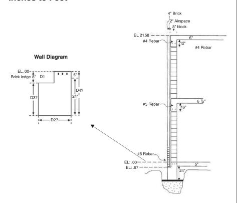
The drawing shown represents the cross section of a two-story building. A cross section shows a view of the internal construction of an object or structure. It represents how it looks when cut on a plane.
