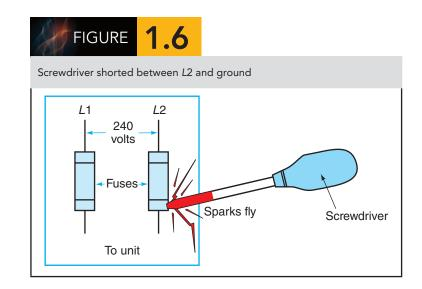
A current flow through the body of 0.015 ampere or less can prove fatal. By comparison, the current draw of a 60-watt light bulb is only 0.50 ampere.
