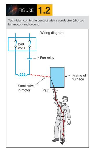
The neutral is a current-carrying conductor in normal operation and is connected to the ground. Another way that you can become part of an electrical circuit is to come in contact with both a conductor supplied with power and with the ground, as shown in **Figure 1.2**. A conductor is a wire or other device that is used as a path for electrical energy to flow. You may become part of the electrical circuit if you touch two conductors supplied with electrical energy, as shown in **Figure 1.3**.
