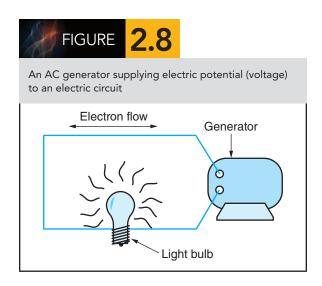
To maintain electric pressure, we must have some way to move electrons in the same manner that water pressure moves water. In an electric circuit, this can be maintained by a battery, as shown in **Figure 2.7** or by a generator or alternator, as shown in **Figure 2.8**. The battery forces electrons to flow to the positive electrode and causes electric pressure. A generator causes electric pressure by transferring electrons from one place to another.
