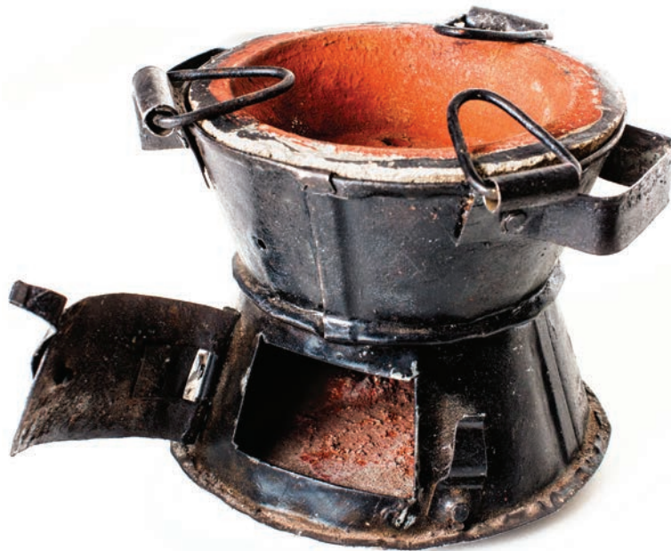
FIGURE 1.13 A Kenyan Jiko . This Kenyan cookstove is made of ceramic and tin and is an improved design that conserves scarce and costly charcoal and wood fuel. The final design resulted from collaboration between those who use them and the Massachusetts Institute of Technology engineers working on the project.
