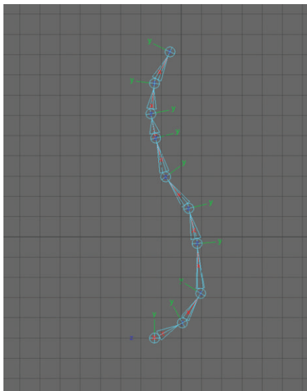
FIGURE 1.26 Local rotation axis set to XYZ on a vertical joint chain, where the axis does not line up from one joint to the next.
