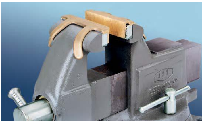
Copper vise-jaw caps can be used to protect vise jaws and surfaces of workpieces from scratching or marring.
