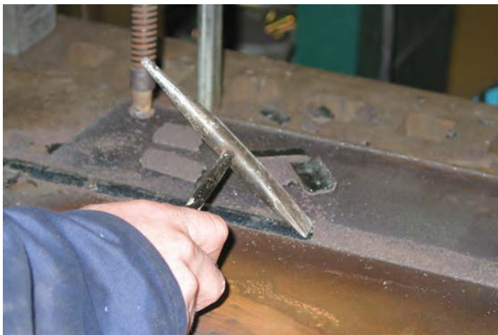
Specialized hammers are used for industrial operations such as removing slag from weld lines.
