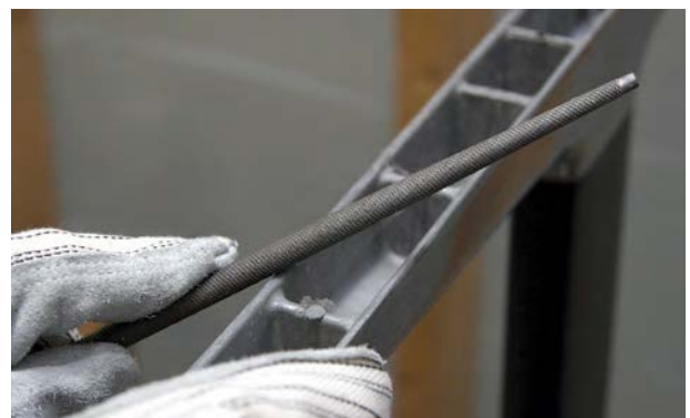
Files are used to remove burrs and rough spots from metal workpieces.
