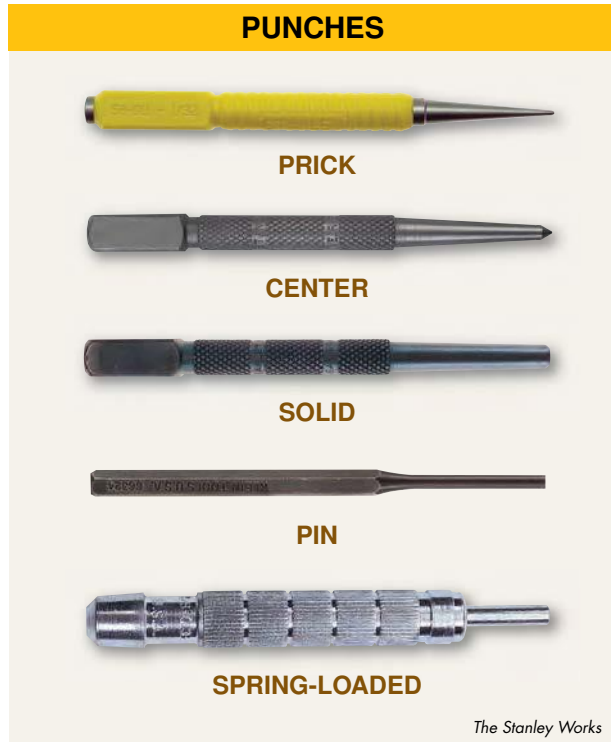
Figure 2-5. A punch is a hand tool with a pointed or blunt tip for marking or making holes or driving objects when struck by a hammer.
