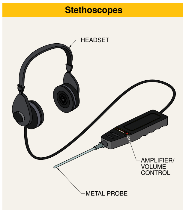
Figure 2-29. Stethoscopes are used for detecting and locating abnormal noises within machines and components.
