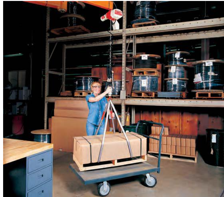
Carts should be used to safely move objects that are heavy or oddly shaped.
