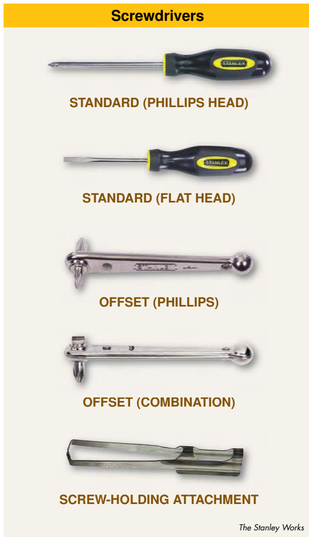
Figure 2-3. Different types of screwdrivers are used for various turning operations.
