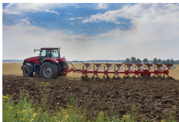
Figure 1.1 Plowing a field. The tractor is pulling a modified moldboard plow, which cuts into the soil, lifts it, and turns it at least partly upside down. This kind of tillage is used less today than it was several decades ago, but it is still in common use around the world.
