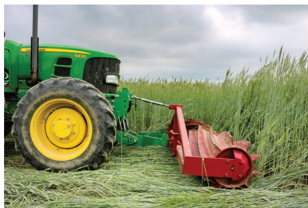
Figure 2.3 A roller crimper. The action of the blades knocks down a cover crop and "crimps" the plants' stems, transforming the crop into a thick, weed-suppressing mulch. Many roller crimpers are designed to be pushed in front of a tractor so that a device behind the tractor can part the flattened mat of stems, drop seeds, and cover them with soil. (Photo courtesy of Rodale Institute.)
