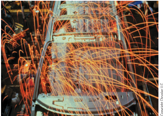
B Unibody vehicles move down an assembly line as automated robots weld the various body panels together.
