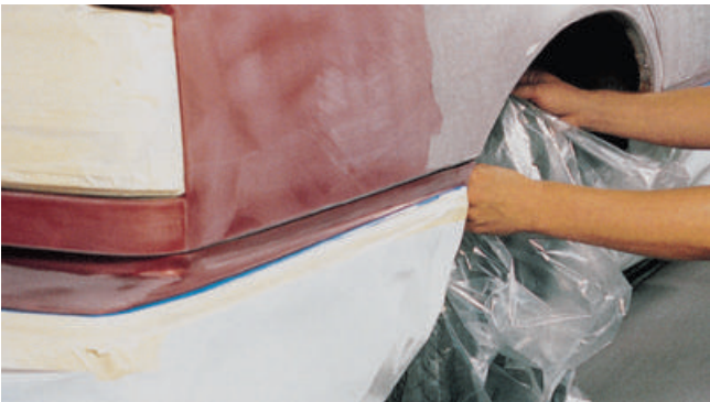
C Plastic wheel masks are installed over tires to protect them from paint spray.
