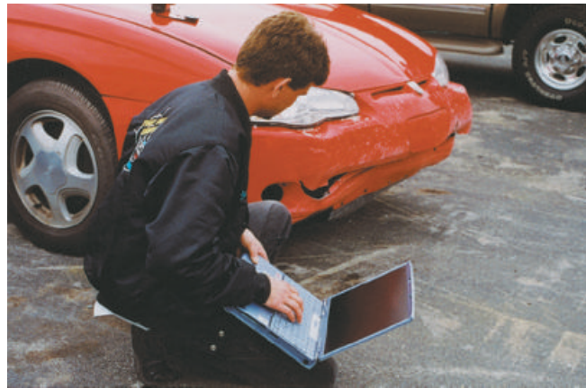
A The estimator must study the damage carefully to determine the cost of repairs. Today's estimators often use an electronic storage unit and electronic camera so that data about damage can be input into the shop's computer.
