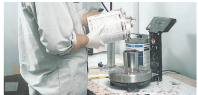
B A computerized electronic scale aids in mixing paint ingredients. Some will give an electronic readout that tells you how much of each ingredient to add while mixing.
