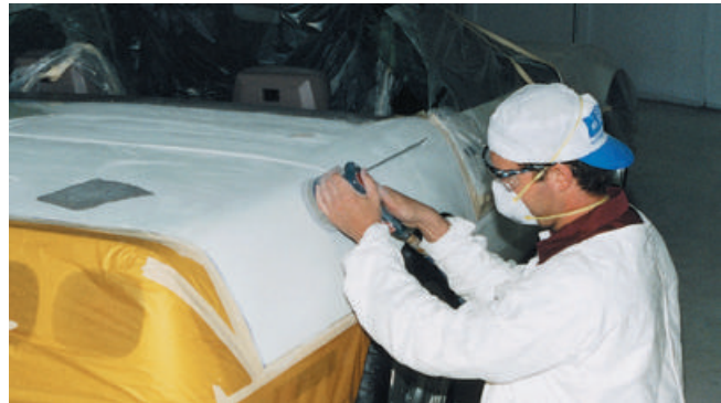
B An orbital sander or hand sanding with fine sandpaper is needed to scuff the old paint to prepare it to accept and bond with the new paint.
