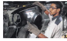
Figure 1-8 To start work, you must normally remove damaged outer body parts to gain access to hidden parts that require straightening or replacement. Here the technician is removing a front fender.
