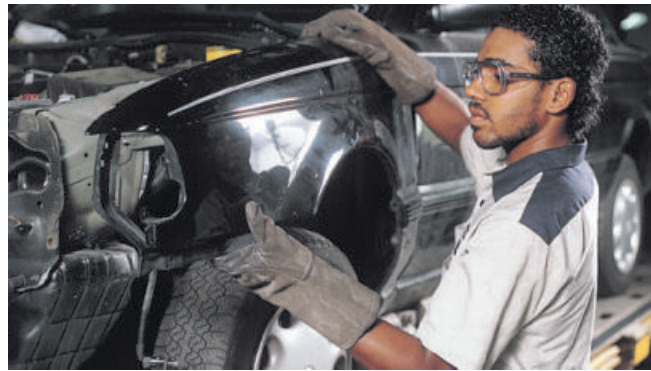
Figure 1-8 To start work, you must normally remove damaged outer body parts to gain access to hidden parts that require straightening or replacement. Here the technician is removing a front fender.
