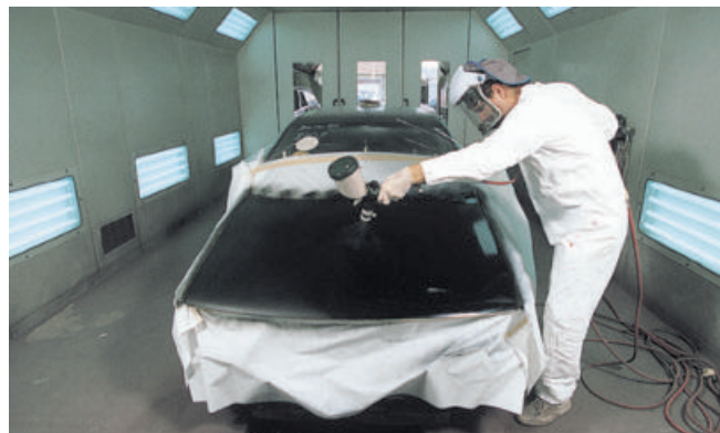
Figure 1-29 Excellent hand-eye coordination and specialized knowledge is needed to be a professional painter. (A) When painting a vehicle, keep the gun the correct distance from the surface. Also keep the gun parallel with the surface. (B) When painting, try to move the spray gun smoothly and evenly. Use straight line paint strokes that overlap evenly. If you move the gun at different speeds or move it further or closer to the surface, paint problems will result.
