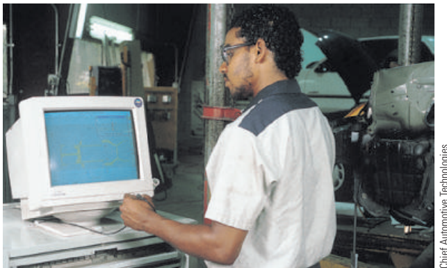
B Computers can quickly compare known good specifications with laser measurements to calculate whether any section of a vehicle has been pushed out of alignment by a collision.
