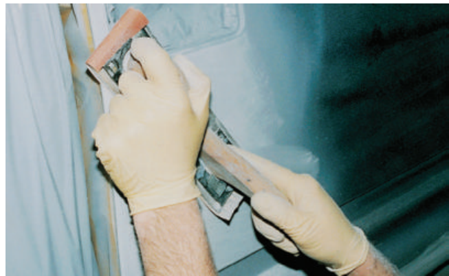
A A large sanding board is commonly used to smooth and level the repair area with the surrounding undamaged areas.
