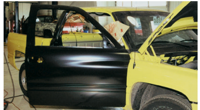
Figure 1-16 Here the entire door frame and skin had to be replaced because it was too damaged to be repaired.
