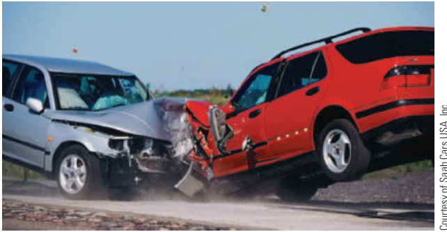
Figure 1-1 During a major collision, like this head-on crash test, tremendous energy is dissipated into the body/frame structures of both cars. Modern vehicles are designed to absorb this energy by controlled collapse of structural body/frame members. The front and rear ends of the vehicles are designed to crush or collapse while keeping the passenger compartment intact. With today's front and side air bags and seat belts, the drivers and passengers would suffer little or no injury in this violent collision.
