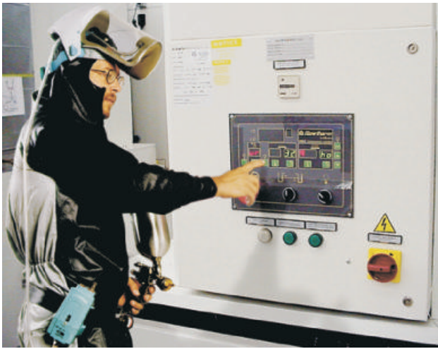
Figure 1-27 Refinish technicians must wear safety gear and be highly skilled at using painting tools and equipment. Here the technician is turning on the fans in a paint spray booth.
