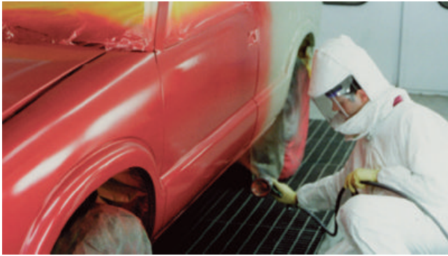
Figure 1-30 Here a refinish technician is spraying the colorcoat along the bottom and side of the car body. This will be followed by spraying the clearcoat to bring out the gloss or shine.
