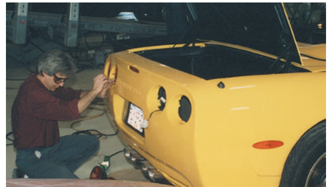
Figure 1-31 After the car body is painted, parts must often be reinstalled. Here a technician reinstalls taillights on this late model sports car.
