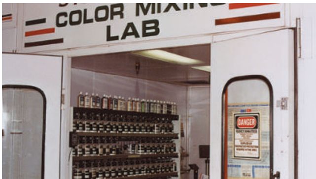
Figure 1-25 Most large body shops have their own paint mixing room. It has all color pigments and other ingredients for mixing paint materials. Mixing rooms also have forced ventilation to prevent buildup of paint fumes.
