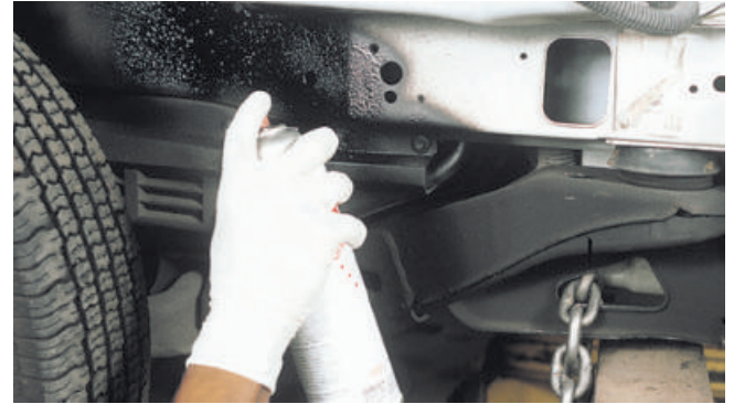
Figure 1-15 You must restore corrosion protection to all repair panels. Various products are available to prevent corrosion or rusting of new panels.
