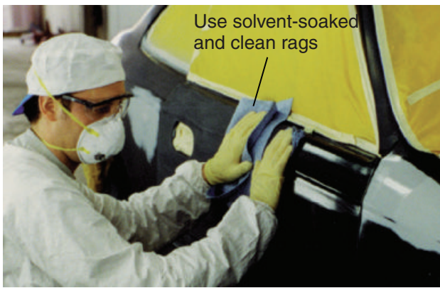
Figure 1-24 Before painting, use two rags to wipe the repair area clean. First, use a rag soaked with wax and grease remover to remove any surface contaminants. Then use a clean rag to wipe the surface while the solvent is still wet.
