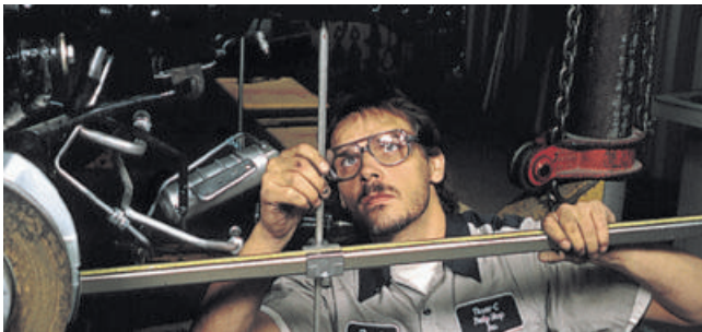
C After tack welding a part, measure its location before final welding. You may need to adjust a part's position while it is still tacked in place.
