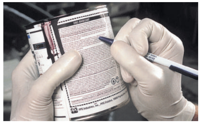
A Mix paint according to label directions or instructions given on the manufacturer procedure sheet. The label or procedure sheet gives ratios for reducer, catalyst, and paint.
