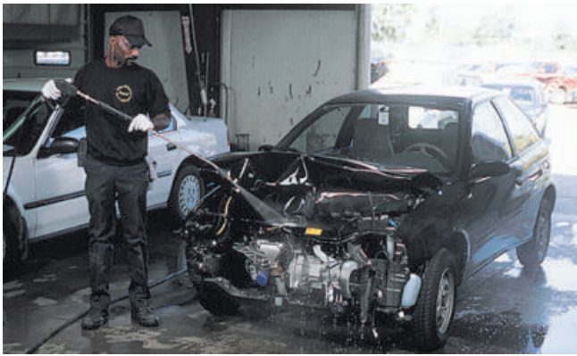
Figure 1-7 Before starting repairs, body shops usually wash the vehicle thoroughly to remove road dirt. Keeping the shop clean is important to refinishing quality because it keeps paint contaminants out of the shop work areas.
