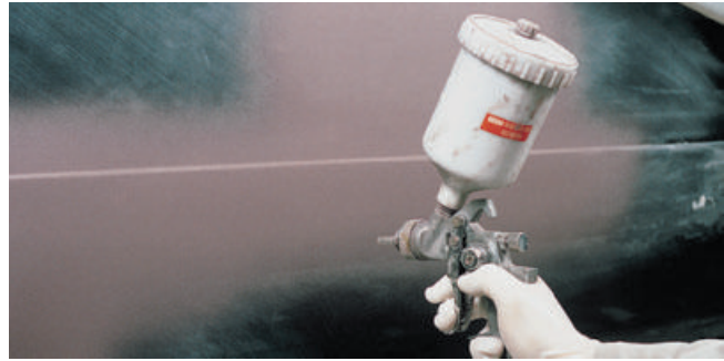
Figure 1-22 Self-etch or epoxy primer must be sprayed over all bare metal to bond to the metal. Primer-surfacer is often sprayed over body filler and the repair area to help level the repair area. Allow each coat of primer to flash properly before applying the next coat.
