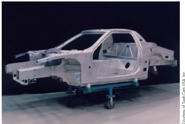
Figure 2-7 Unibody vehicles consist of small body panels welded together to serve as the vehicle frame. Unibody vehicles are light yet very strong. They are built for controlled collapse during a collision to help keep the passenger compartment intact.
