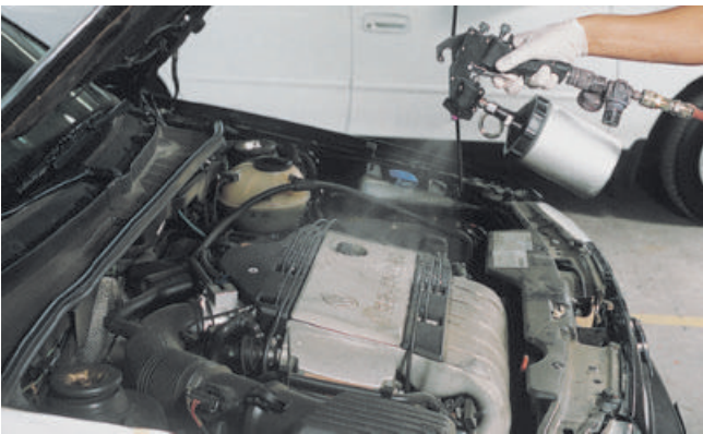
B Spray-on masking material is handy when masking a large area, such as underhood components. It is water-based masking coating and can be washed off with soap and water after painting.
