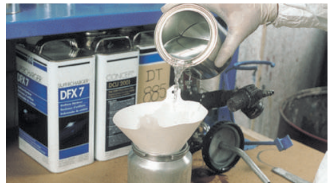
C Filter everything that goes into the spray gun cup. One piece of dirt or cured paint can ruin a paint job.
