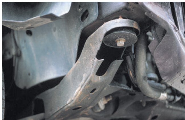
C Damage to the engine, engine mounts, pulleys, and underbody parts must be accounted for in an estimate. Sometimes the vehicle is raised on a lift for undercarriage inspection.
