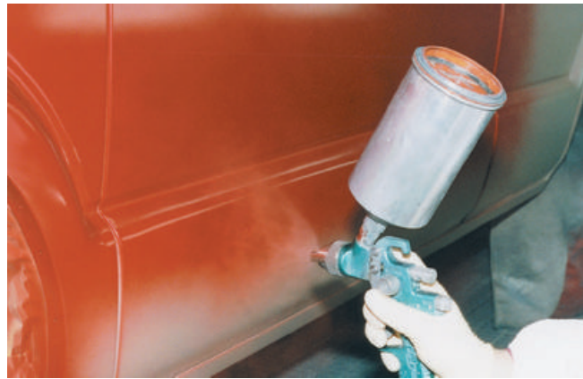
Figure 1-28 The spray gun is the main tool of a body shop paint technician. It must be adjusted properly to produce a smooth, even paint film on the vehicle.
