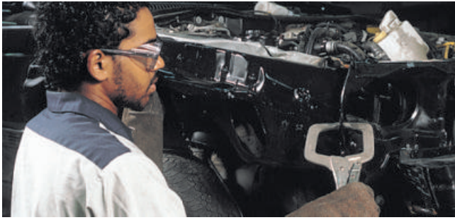
A New structural parts must be temporarily held in place with clamping pliers or screws.
