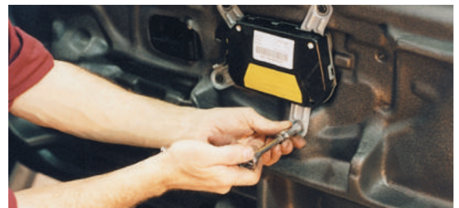
Figure 1-17 A technician replaces a small air bag located on the inside of the door frame. Note how the technician stays to one side in case the air bag accidentally deploys. Air bags deploy with a “bang” and can cause injury to your arms, hands, and face.
