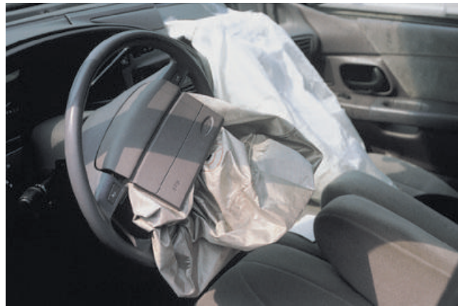
B The vehicle interior is often damaged in a major collision. Replacing deployed air bags is expensive and must be included in the estimate.
