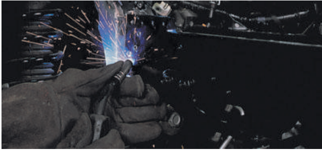
B First, tack weld parts in place, using only a few welds to hold the parts in alignment.
